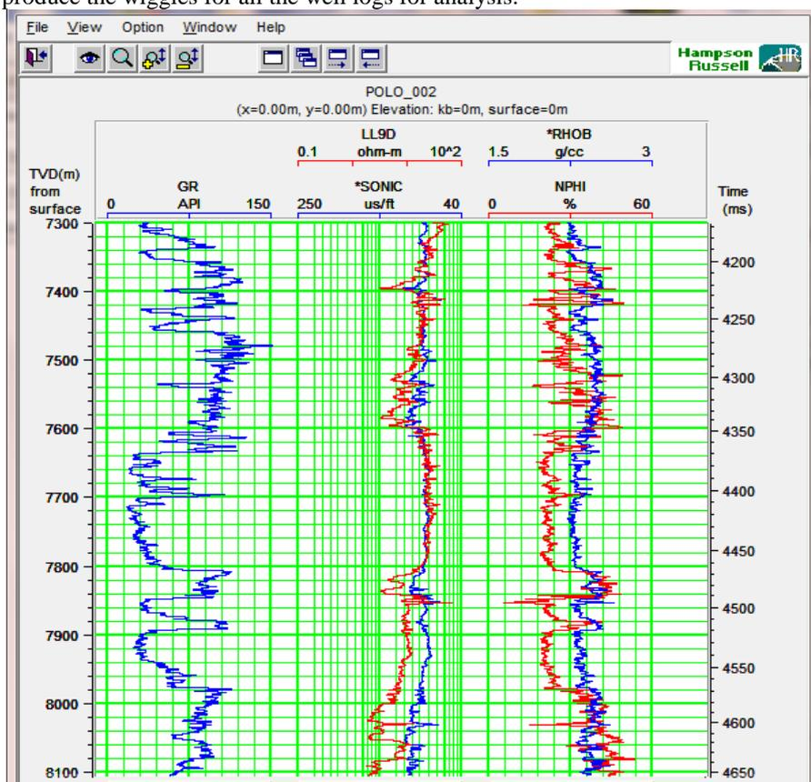
Figure 4: Composite log plot in Geoview showing the wiggles (track) display for all the well logs.
