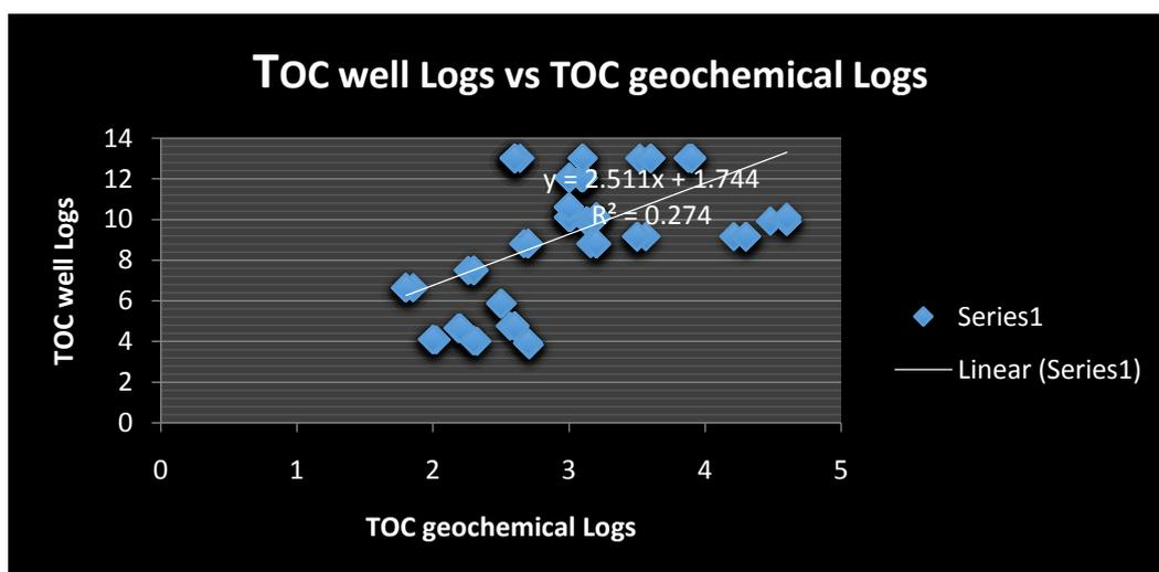
**Figure 8:** TOC well Logs vs TOC geochemical Logs. The graph shows the level of deviation between the two data set, however the deviation level is still within acceptable limits of error, hence the TOC estimated from well log is reliable
