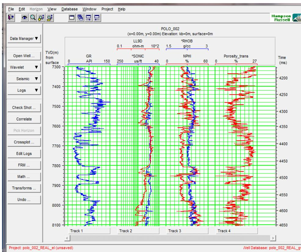
**Figure 5:** Composite log track showing porosity log (track 4) derived from density. The red circle shows the curve separation ( $\Delta\log R$ ) or Sonic-resistivity overlay at a depth of 7820 – 7840(ft).
