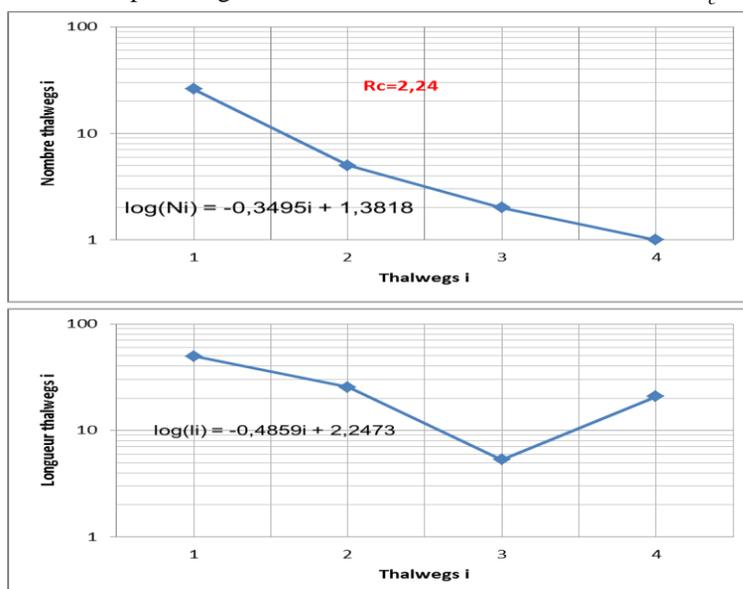
Figure 10: Laws of Horton applied to the catchment area of Kinsenda
