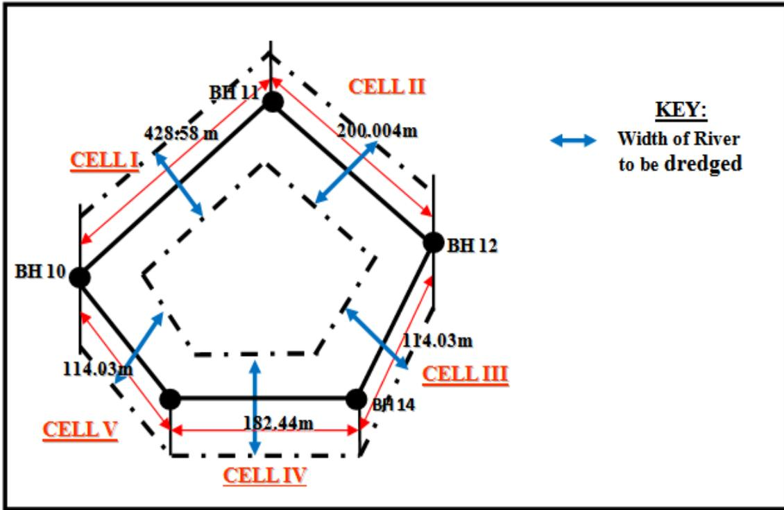
APPENDIX A 2: Schematic Cross-Section of the Project Site Showing Boring Locations, Actual Distances and Approximate Width of Creeks at Borrow Pit 'B'
