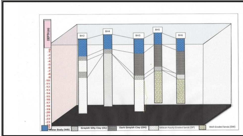
Figure 3b: Fence Diagram of Strata Logs at Borrow-Pit B
