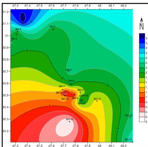
Figure 1.9: The horizontal distribution of the organic matter from the fifth- meter depth of the study area soils.
