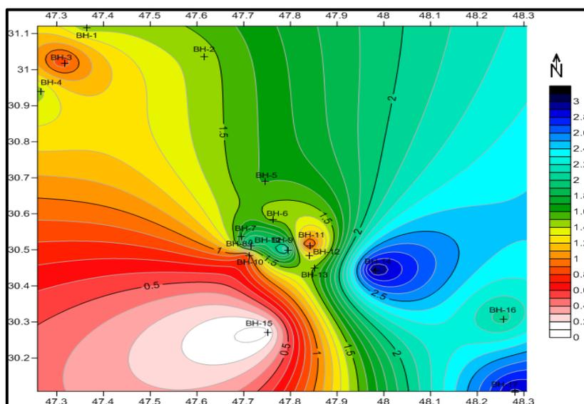
Figure 1.5: The horizontal distribution of the organic matter from the first-meter depth of the study area soils.
