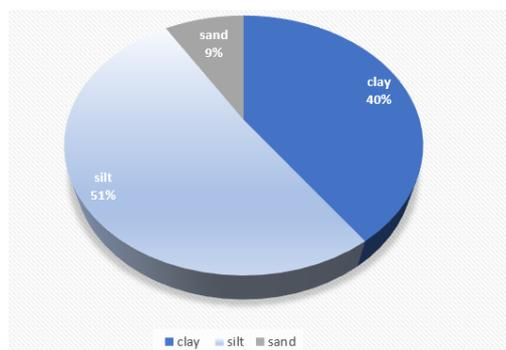
Figure 1.2: The results of grain size analysis test for studied soils.
