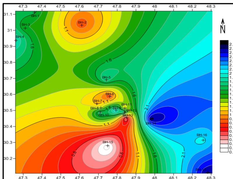
Figure 1.6: The horizontal distribution of the organic matter from the second-meter depth of the study area soils.
