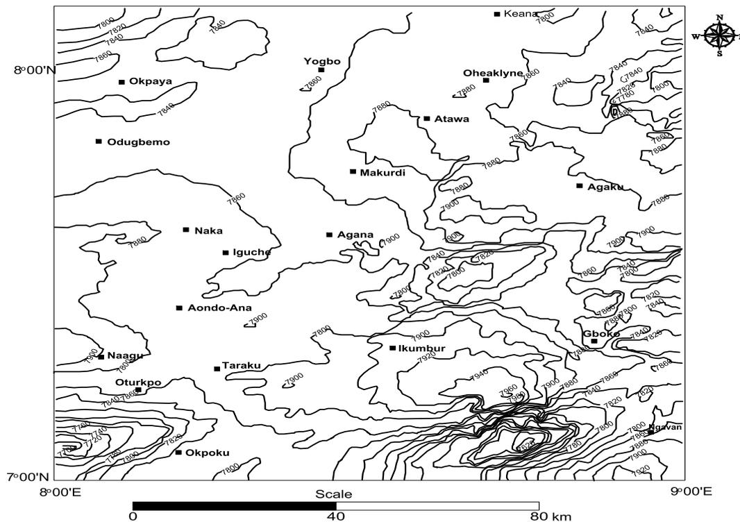
**Fig. 3: Total Magnetic Field over the Study Area as Contour Map (Contour interval = 20nt)**
