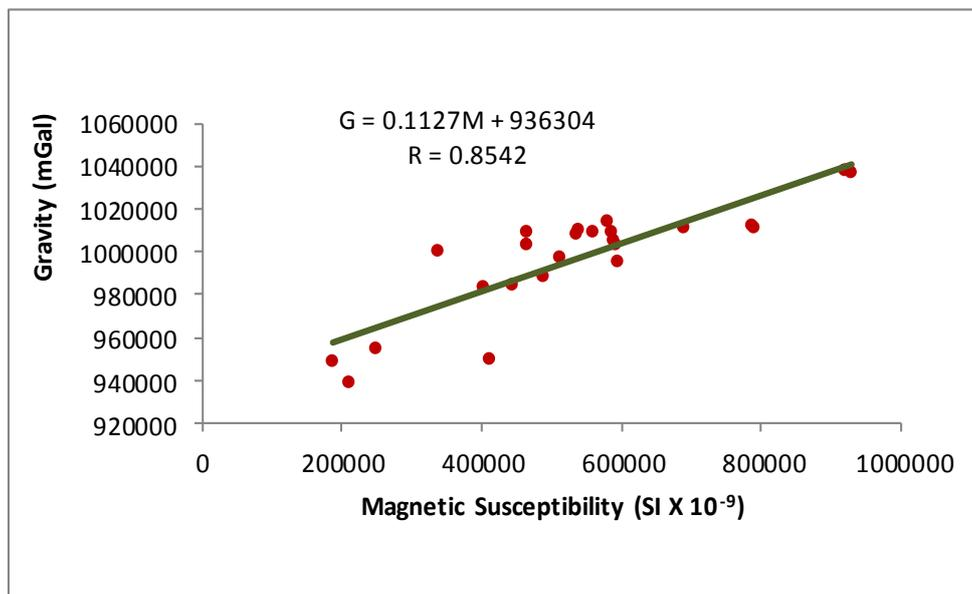
Figure 7: Crossplot of the Magnetic Susceptibility(M) and Gravity (G)
