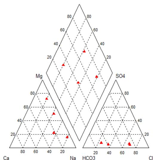
Figure 3: The Piper plot of the Tista riverwater
