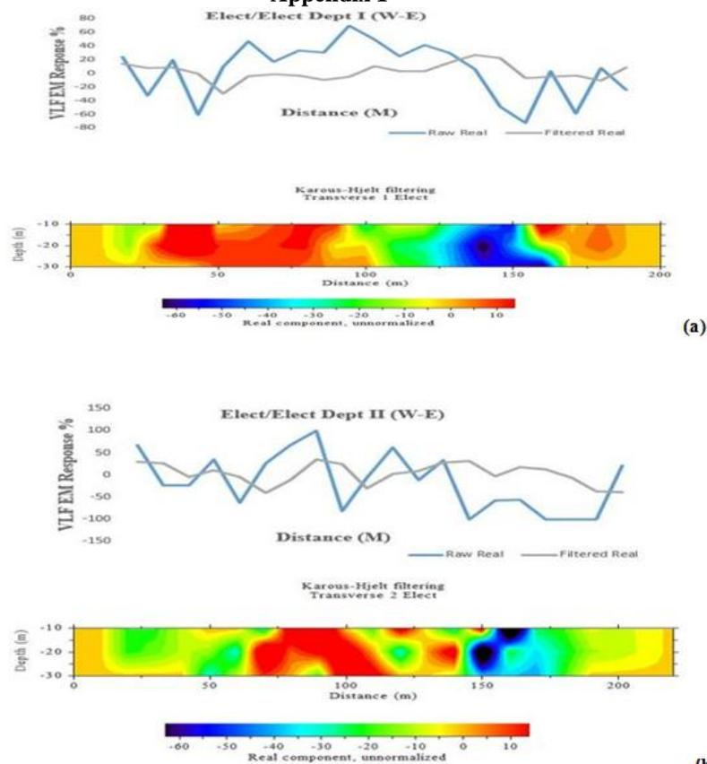
**Figure 5:** Plot of VLF results along the profile 5 ( $T_9$  a, and  $T_{10}$  b), unfiltered Real component of VLF-EM data, Fraser filtered real (in-phase) data against distance, and Karous and Hjelt pseudo-section of in-phase data (apparent current density pseudo-section) against distance.
