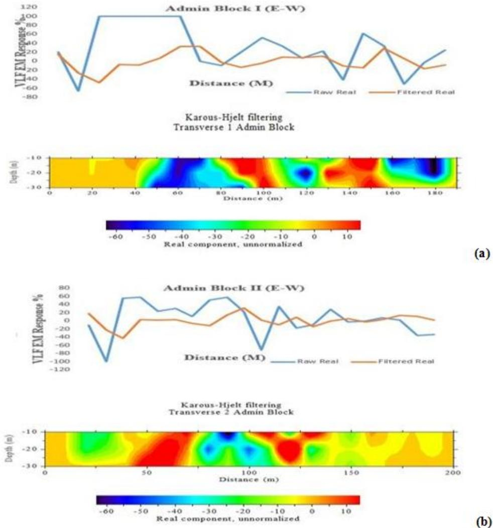
**Figure 2:** Plot of VLF results along the profile 1 ( $T_{1a}$ , and  $T_{2b}$ ), unfiltered Real component of VLF-EM data, Fraser filtered real (in-phase) data against distance, and Karous and Hjelt pseudo-section of in-phase data (apparent current density pseudo-section) against distance.
