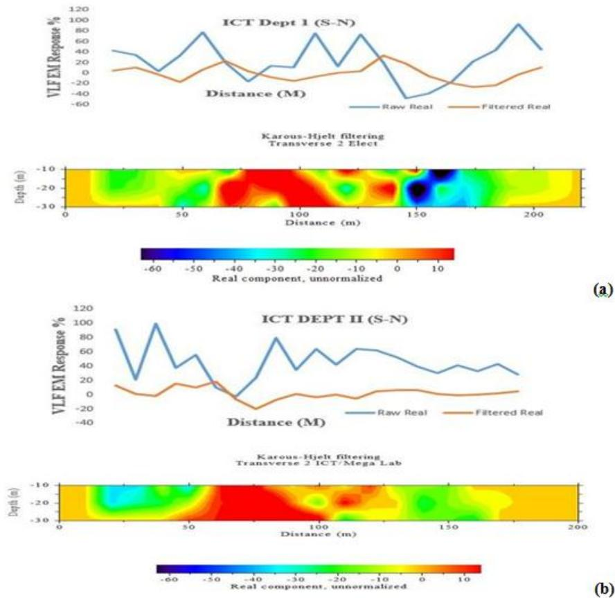
Figure 7: Plot of VLF results along the profile 6 ( $T_{11}$  a, and  $T_{12}$  b), unfiltered Real component of VLF-EM data, Fraser filtered real (in-phase) data against distance, and Karous and Hjelt pseudo-section of in-phase data (apparent current density pseudo-section) against distance.
