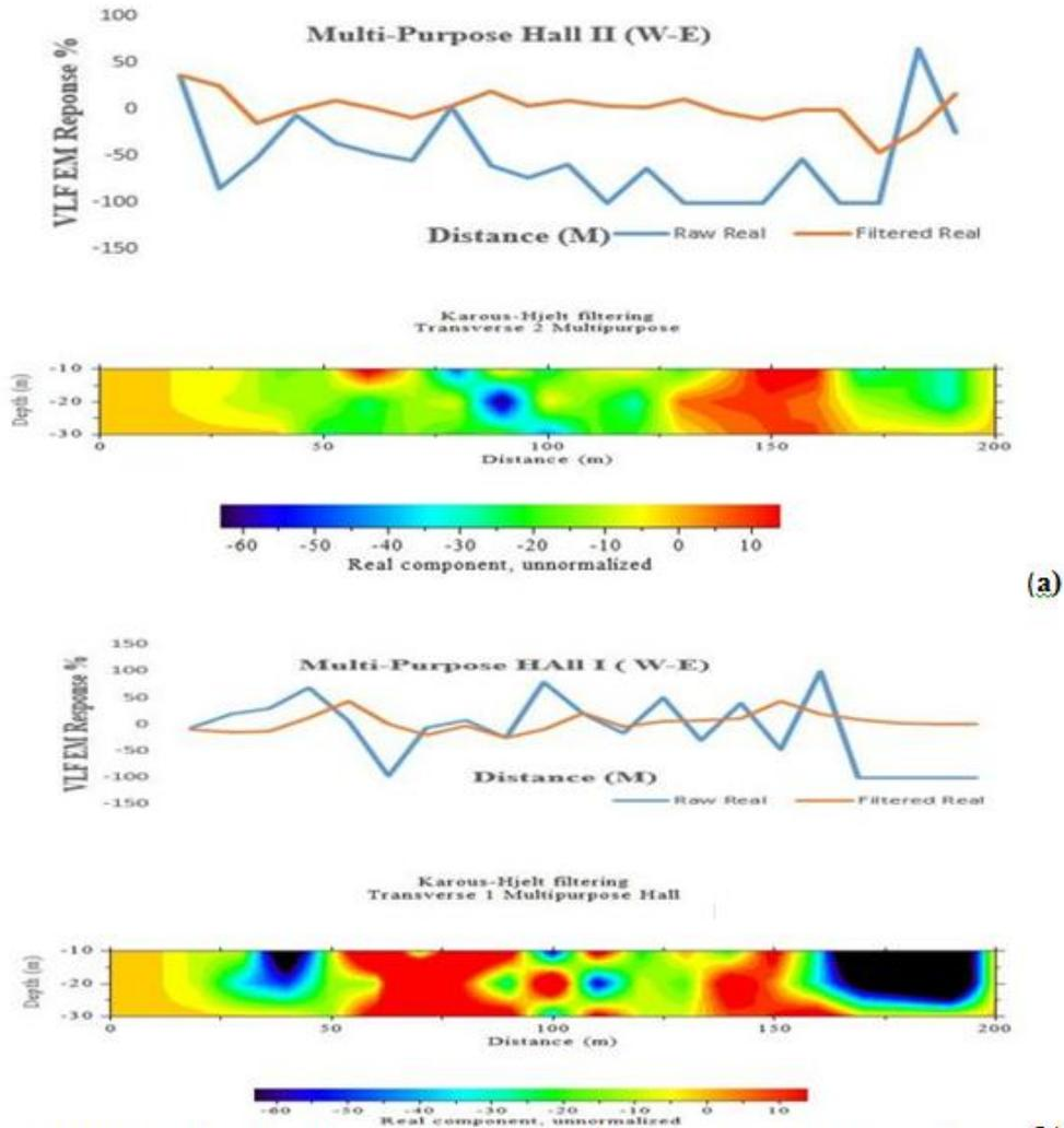
**Figure 3:** Plot of VLF results along the profile 2 (T<sub>3a</sub>, and T<sub>4b</sub>), unfiltered Real component of VLF-EM data, Fraser filtered real (in-phase) data against distance, and Karous and Hjelt pseudo-section of in-phase data (apparent current density pseudo-section) against distance.
