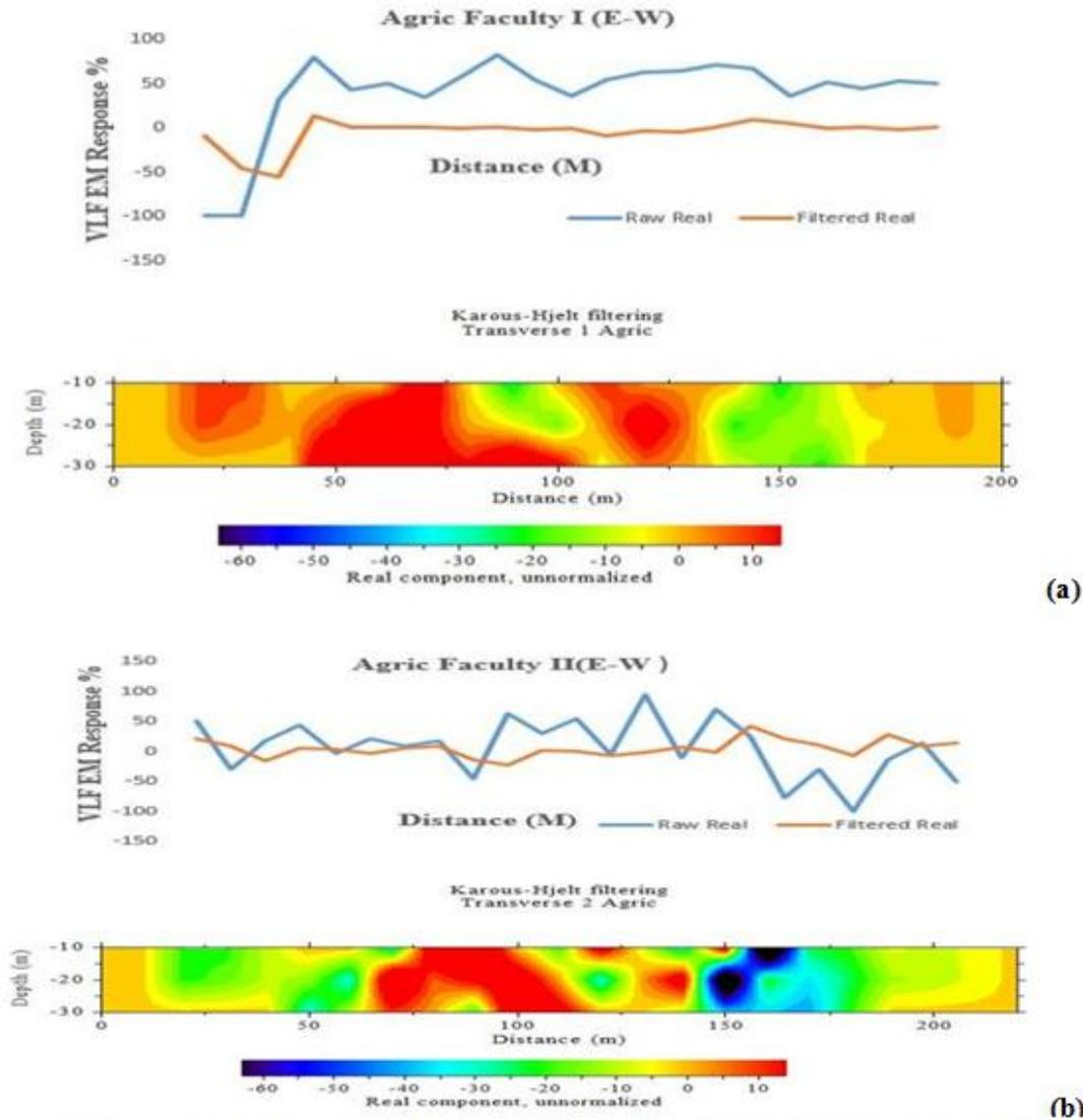
**Figure 5:** Plot of VLF results along the profile 4 ( $T_7$  a, and  $T_8$  b), unfiltered Real component of VLF-EM data, Fraser filtered real (in-phase) data against distance, and Karous and Hjelt pseudo-section of in-phase data (apparent current density pseudo-section) against distance.
