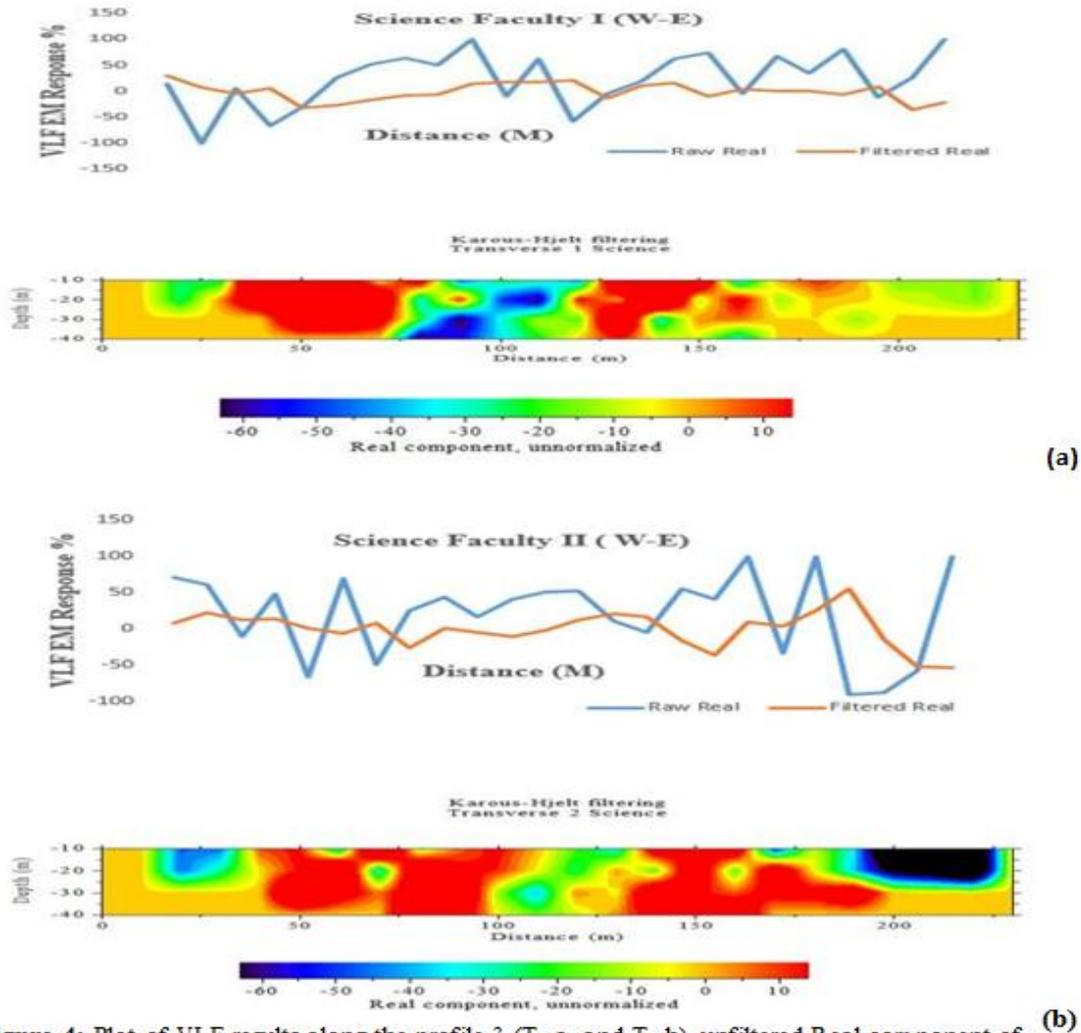
**Figure 4:** Plot of VLF results along the profile 3 ( $T_5$  a, and  $T_6$  b), unfiltered Real component of VLF-EM data, Fraser filtered real (in-phase) data against distance, and Karous and Hjelt pseudo-section of in-phase data (apparent current density pseudo-section) against distance. (b)
