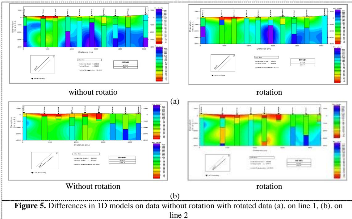
Figure 5. Differences in 1D models on data without rotation with rotated data (a). on line 1, (b). on line 2
