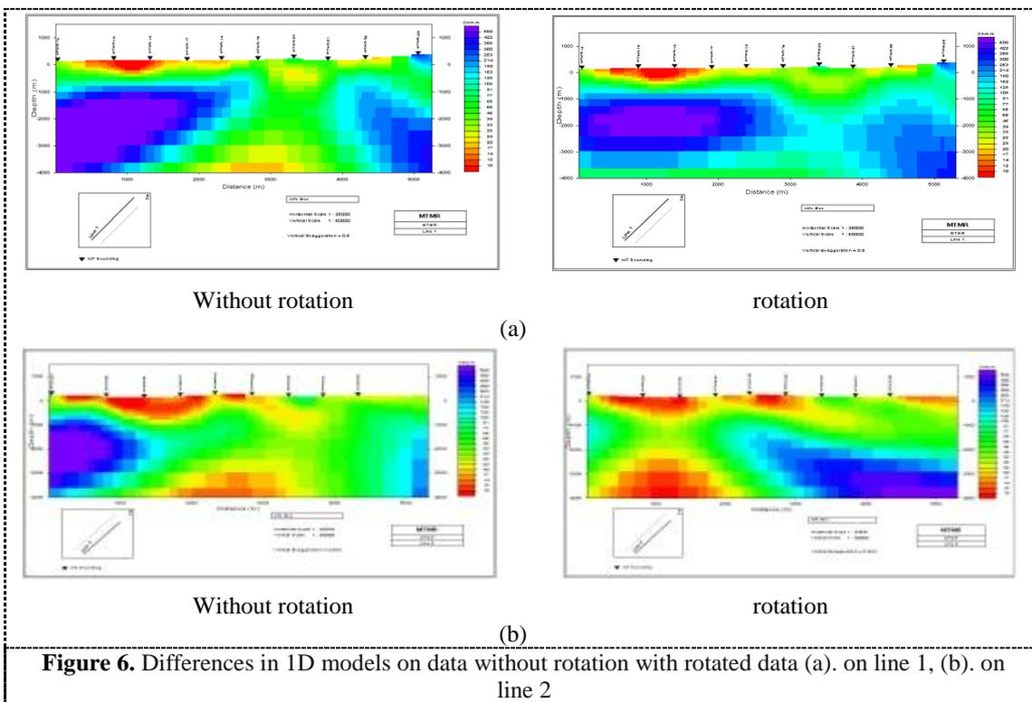
Figure 6. Differences in 1D models on data without rotation with rotated data (a). on line 1, (b). on line 2
