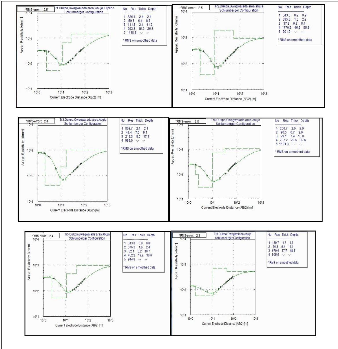
Table 4 is a summary of the interpretation of the results of the Vertical Electrical Sounding in the study area. The results show that the area is characterized by 4 to 5 geoelectric subsurface layers.
