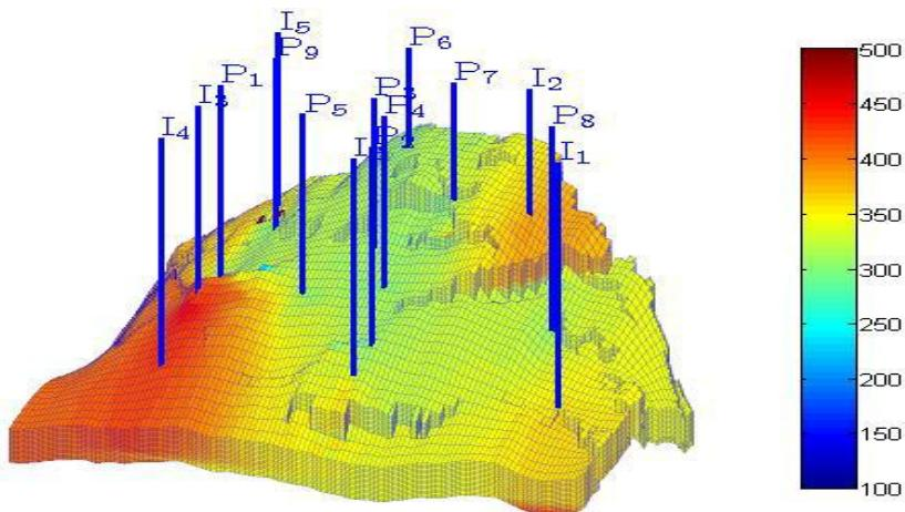
**Figure 4:** Geologic model showing initial pressure distribution measured in bar
