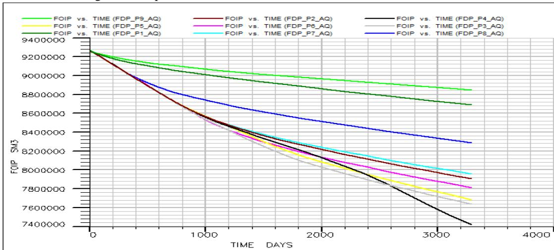
**Figure 11:** A plot showing field oil in place, before, during and after production
