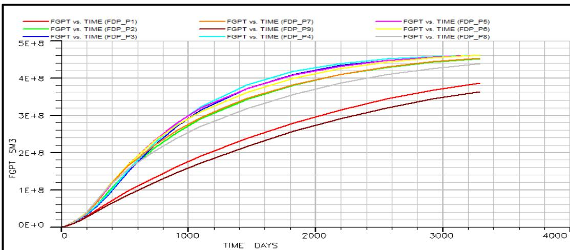
**Figure 7:** Graph showing cumulative gas production without aquifer for all the 9 wells
