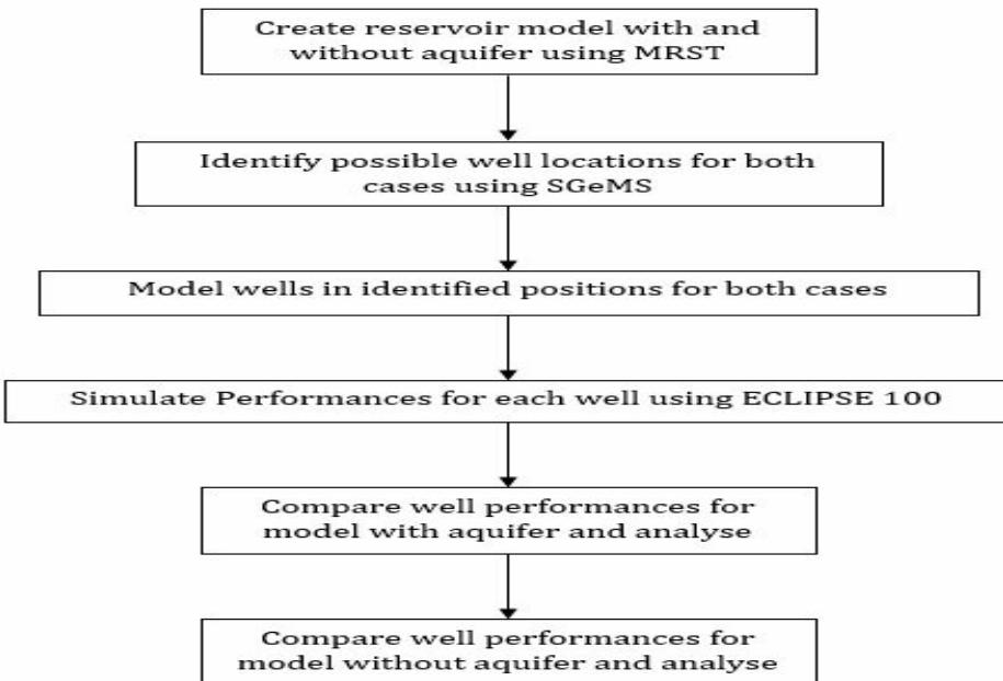
**Figure 2:** Flow chart indicating the step by step process carried out
