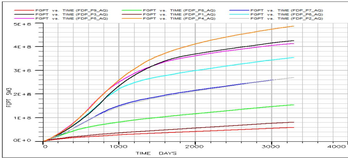
**Figure 12:** Plot showing gas production from the nine (9) wells
