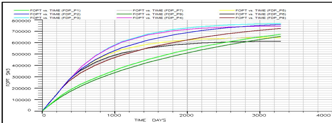
**Figure 6:** Graph showing cumulative oil production without aquifer for all the 9 wells.
