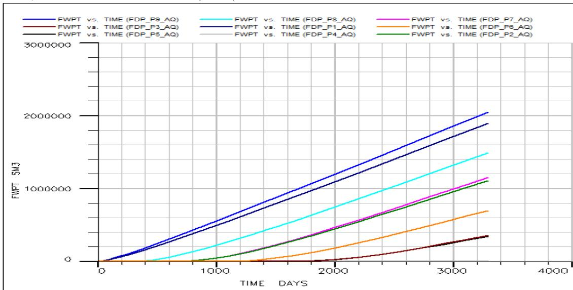
**Figure 13:** Plot showing water production from the nine (9) wells
