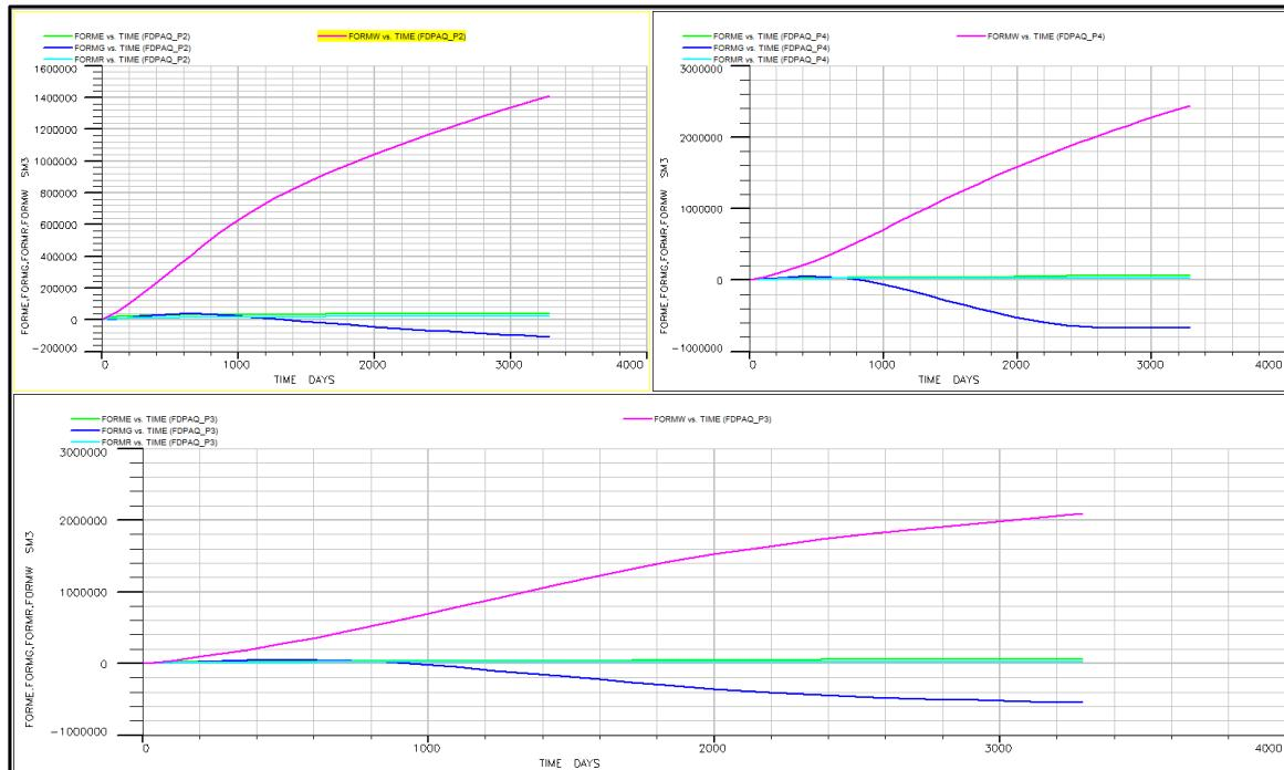
**Figure 14:** Plot showing the major drive mechanisms per well with aquifer
