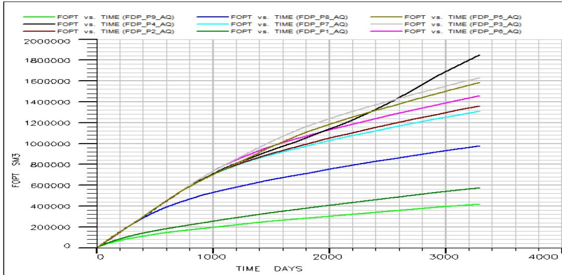
**Figure 10:** Plot cumulative oil production per wells with aquifer
