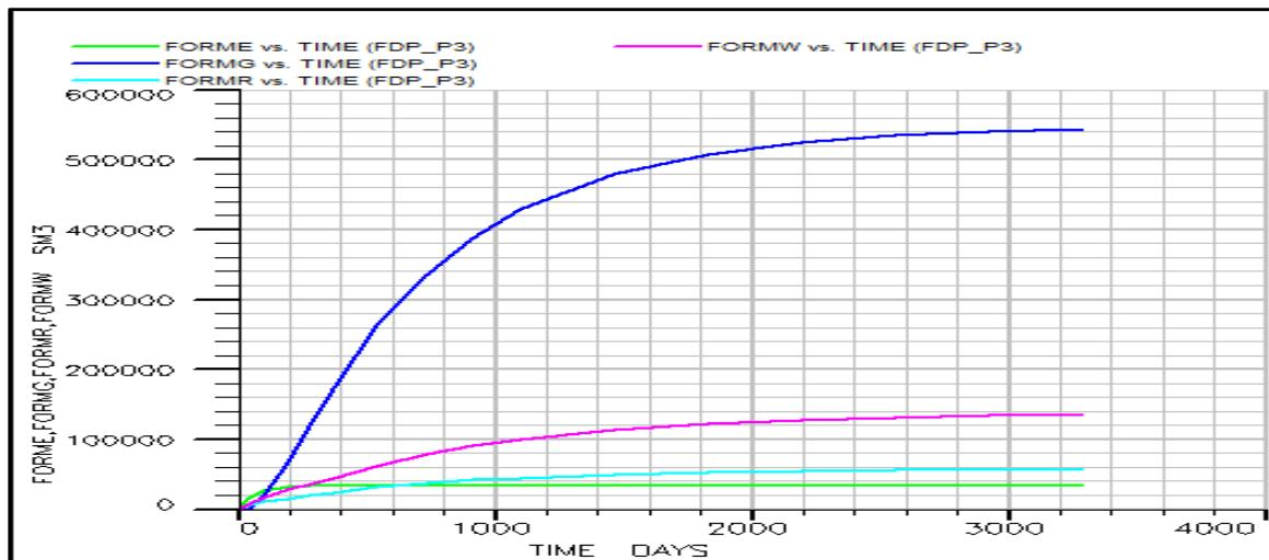
**Figure 9:** Graph showing the four major drive mechanisms contributing to the production of oil in well 3
