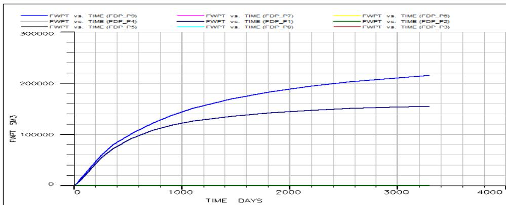
**Figure 8:** Graph showing cumulative water production without aquifer for all the 9 wells
