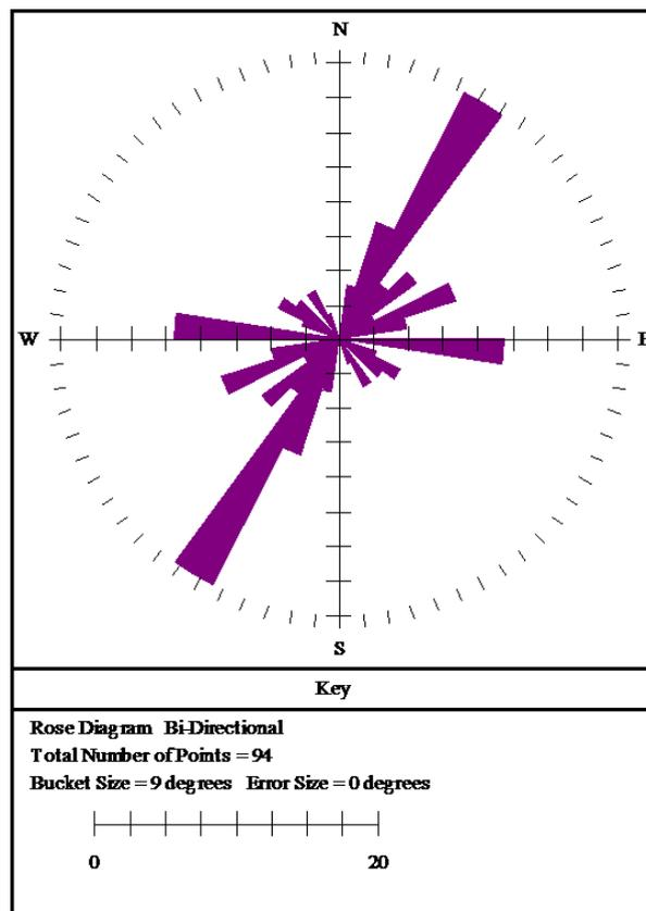
Figure 6: Rose diagram showing orientation of lineaments of the study area
