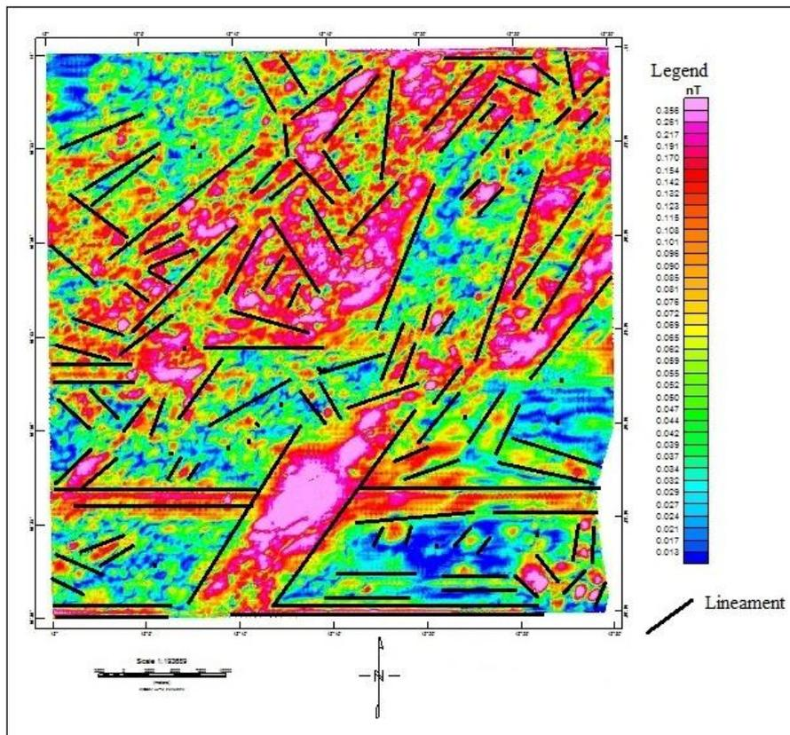
Figure 5: Analytic Signal Map of the Study Area showing Lineaments.
