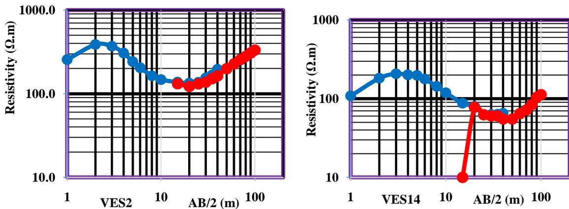
Figure 3: VES curves of recent basalts without pyroclastic cover
