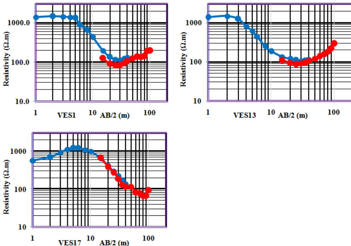
Figure 2: VES curves of recent basalts under weak pyroclastic cover
