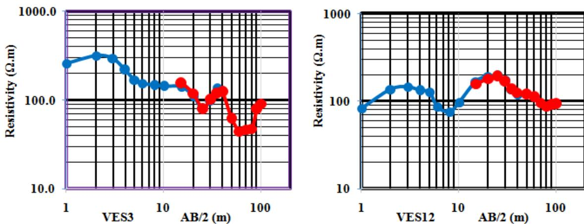
Figure 4: VES curves of recent basalts without pyroclastic covers showing anisotropies
