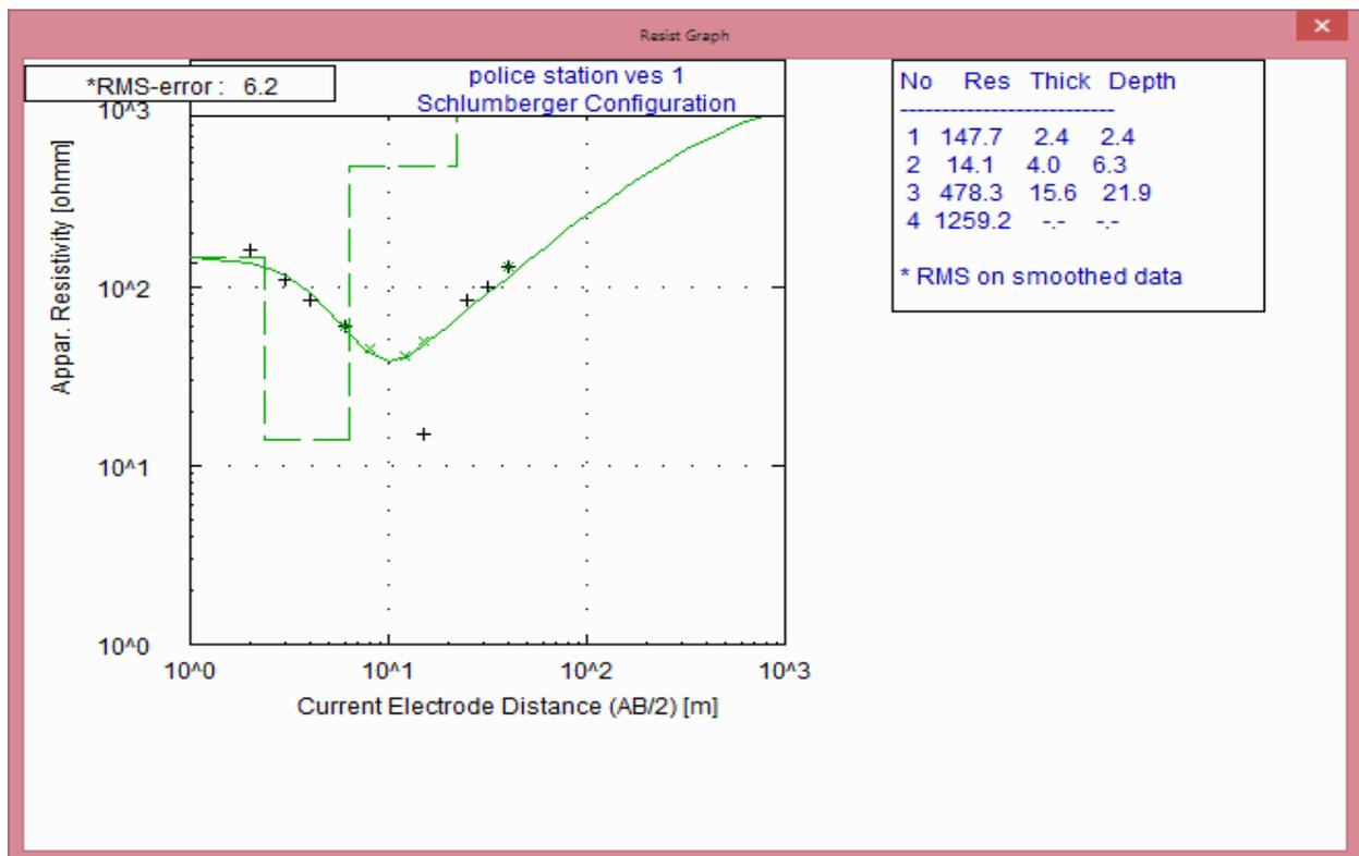
Figure 3. A typical depth sounding curve displaying 1D geoelectric section along a traverse.
