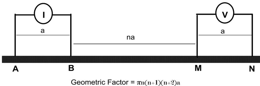
(b) Dipole-Dipole electrode array [22]
