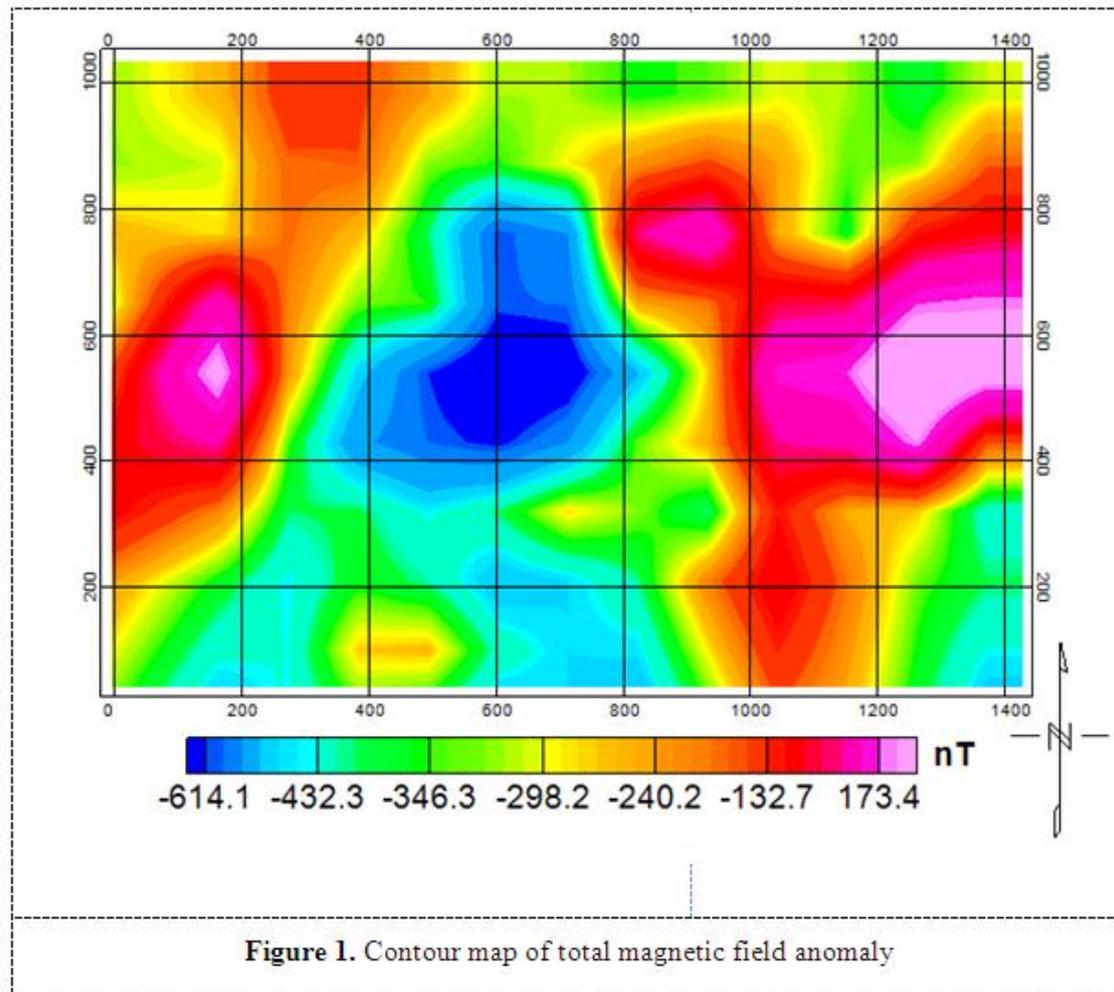
The pattern on the contour of the total magnetic field anomaly consists of positive closure with a maximum value of 373.7 nT and negative closure with a minimum value of -1513.3 nT which indicates that the magnetic field anomaly is a dipole. The magnetic field anomaly is the result of a combination of the raman magnetic field and the induced magnetic field.
