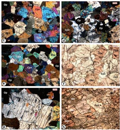
Photomicrographs of Pyroxenite (Thin Section from c,d,e,g) and Granulite (Thin Section from f and h)
