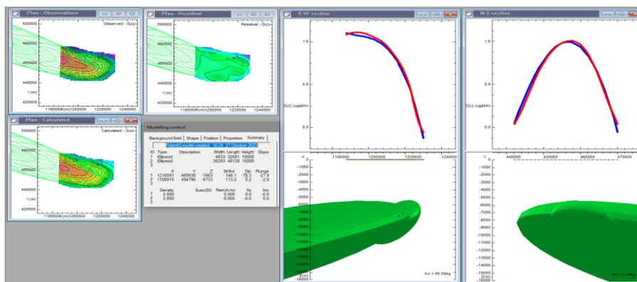
Figure 13. Representation of the subsurface structure of anomaly A6
