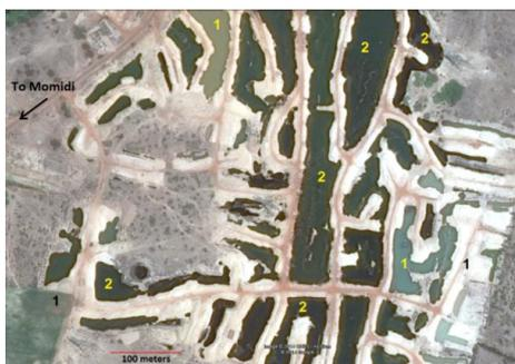
**Figure.2.** Google Earth image showing deeper/idle mines (1) and active/recent mines (2) of Momidi area. Tonal change between old and new excavation can be noticed.
