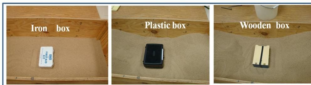
Figure 3: An iron (20 cm length, 13cm wide, and 7 cm high), plastic (22 cm length, 18cm wide, and 10.5 cm high), and wooden (19.5 cm length, 15cm wide, and 9 cm high) boxes filled with iron and copper materials were used as a subsurface targets (weapons and unexploded ordnance).
