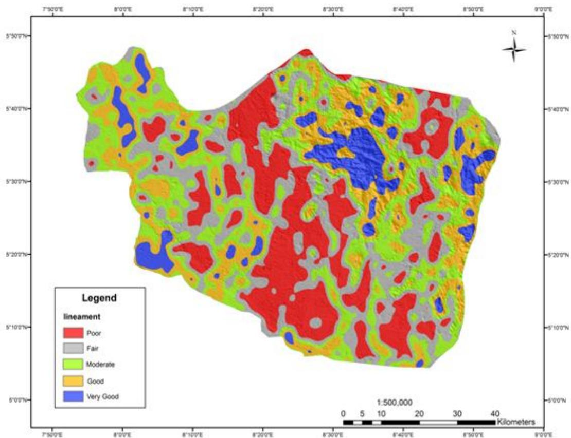
Figure 11. Stability range of lineament density map for groundwater accumulation
