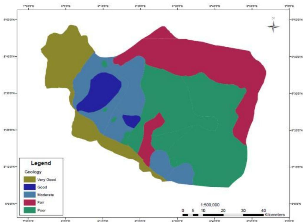
**Figure 13.** Stability range of reclassified geologic map for groundwater accumulation
