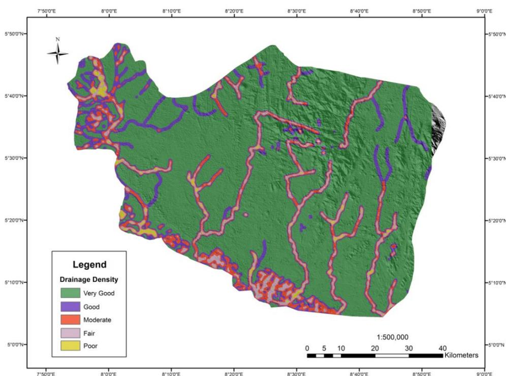
**Figure 9.** Stability range of drainage density map for groundwater accumulation in the study area
