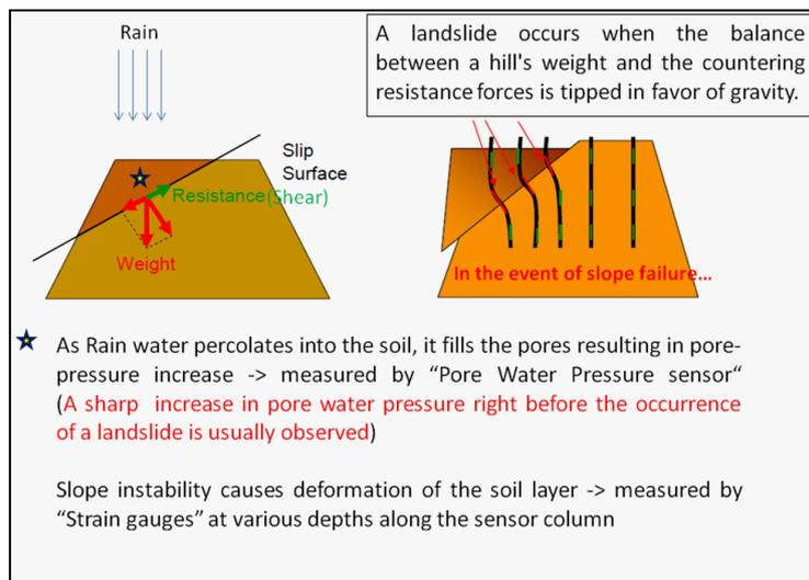
Fig. 1.Slip surface characteristics
