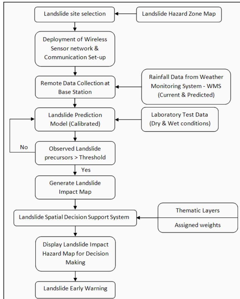
Fig. 2. Proposed Landslide Monitoring and Prediction System (LMPS)
