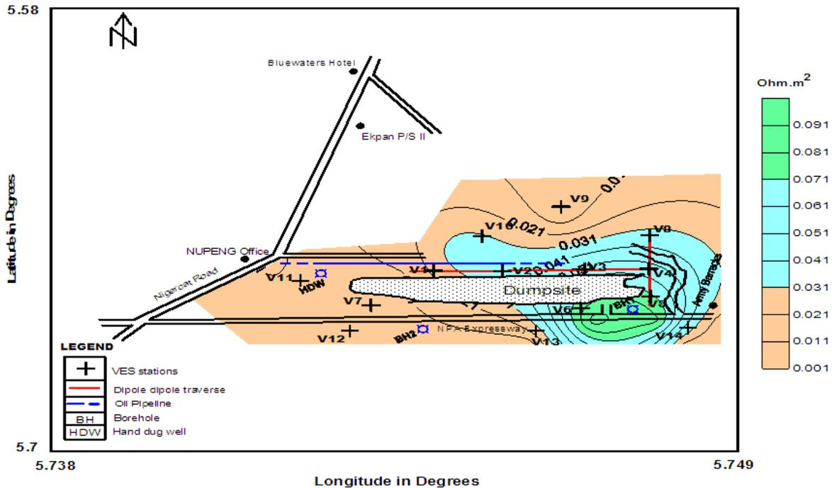
Figure 9: Aquifer protective capacity map over the dumpsite area
