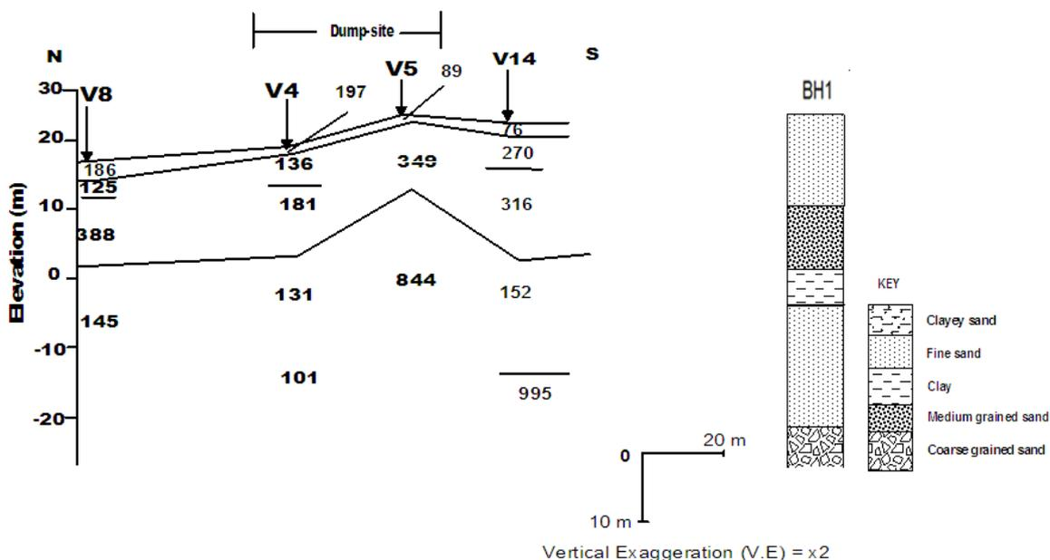
Figure 4: Geoelectric Section along the N-S Direction across the dumpsite area
