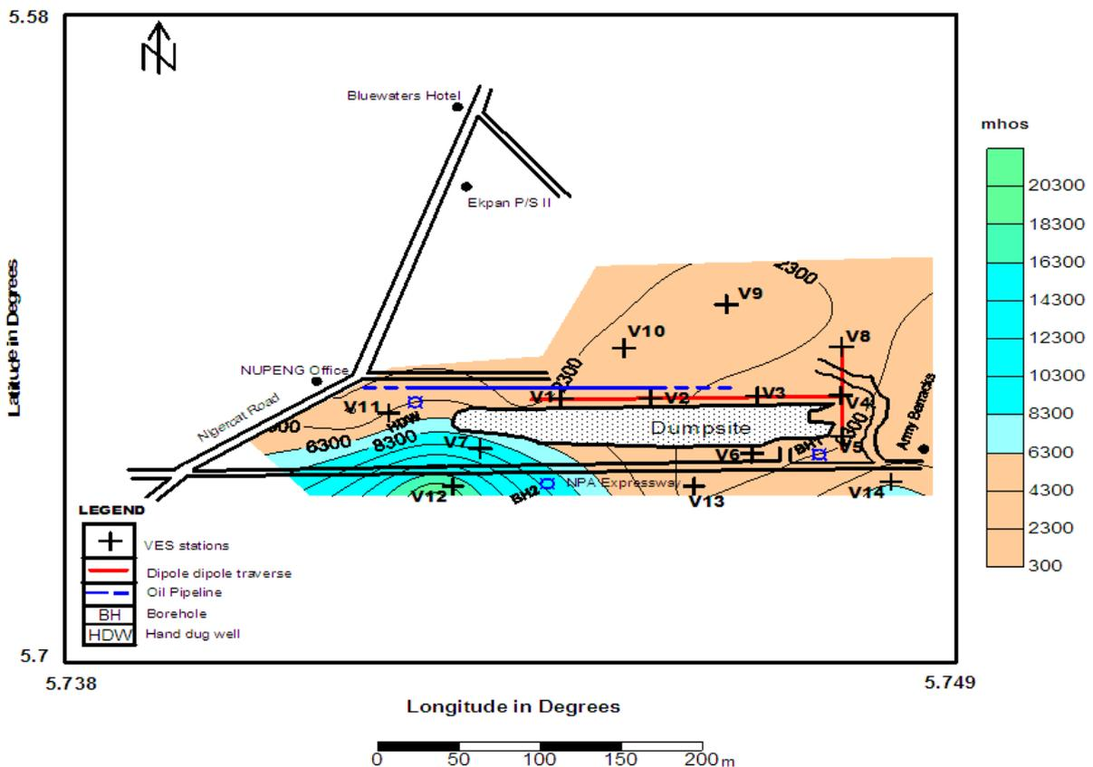
Figure 10: Aquifer transmissivity Map over the dumpsite area
