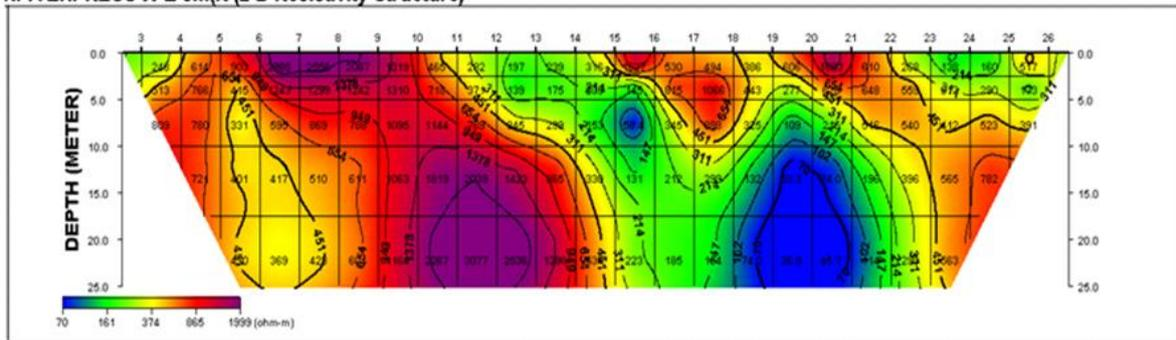
Figure 7: 2-D Resistivity Structure at a= 5 m in the W-E Direction Across the dumpsite area
