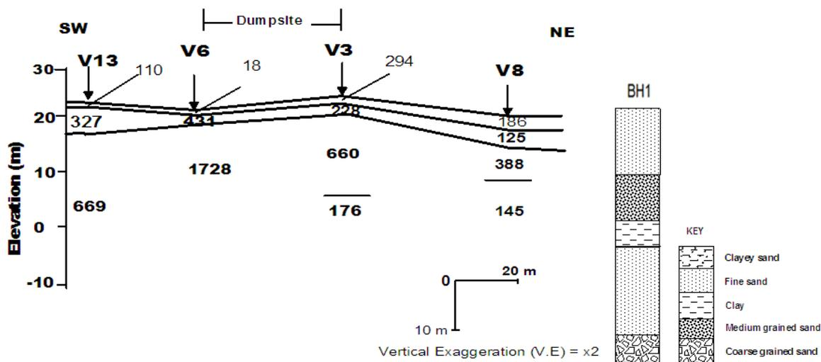
Figure 6: Geoelectric Section along the SW-NE Direction across the dumpsite area
