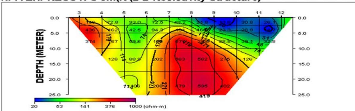
Figure 8: 2-D Resistivity Structure at a= 5 m in the N-S Direction Across the dumpsite area
