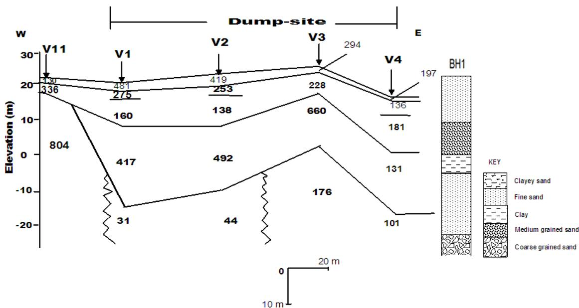
Figure 3: Geoelectric Section along the SW-NE Direction across the dumpsite area
