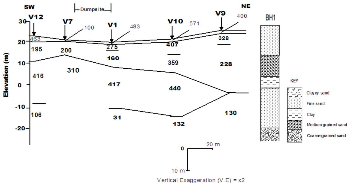
Figure 5: Geoelectric Section along the SW-NE Direction across the dumpsite area
