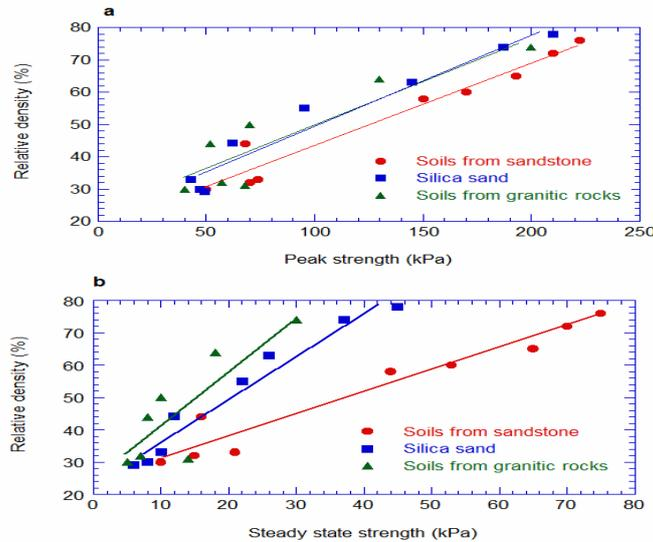
Figures 4a and b: The peak and steady state strength characteristics of the different slope soils
