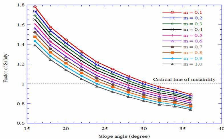
Figure 6: The effect of saturation and slope angle on the factor of safety for slopes on sedimentary rocks
