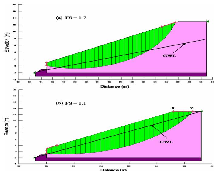
**Figures 8a and b:** Stability analysis using actual ground water levels of the study area
