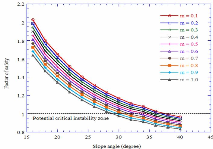
**Figure 7:** The relationship between factor of safety and slope angle for slopes on igneous and metamorphic rocks
