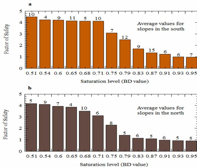
Figures 5a and b: The variation of factor of safety with changing saturation level
