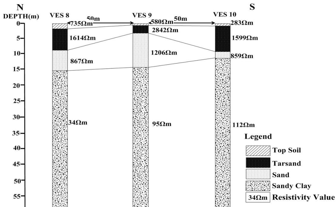
Figure 6: Geo-Electric section along Traverse 2 in Looda village
