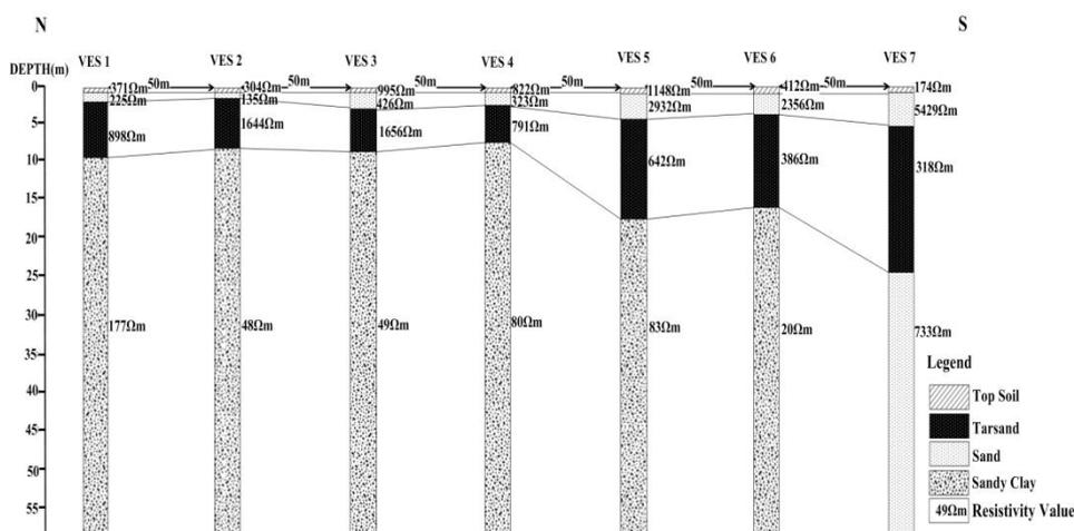
Figure5: Geo-Electric section along Traverse 1 in Looda village
