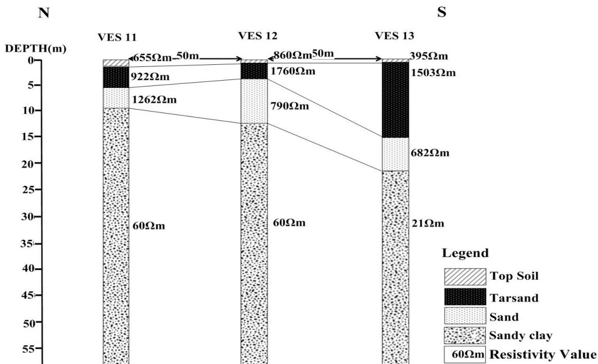
Figure 7: Geo-Electric section along Traverse 3 in Looda village
