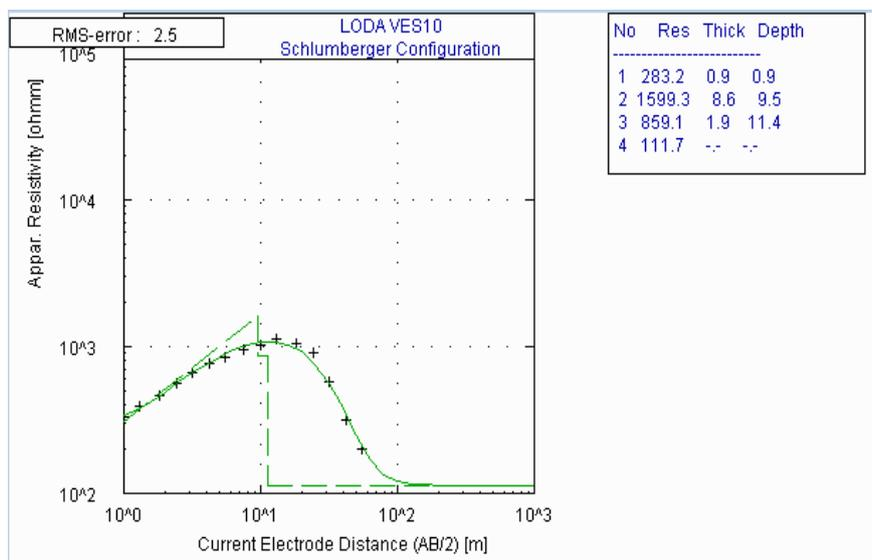
Figure 4c: Typical KQ curve-type in the area
