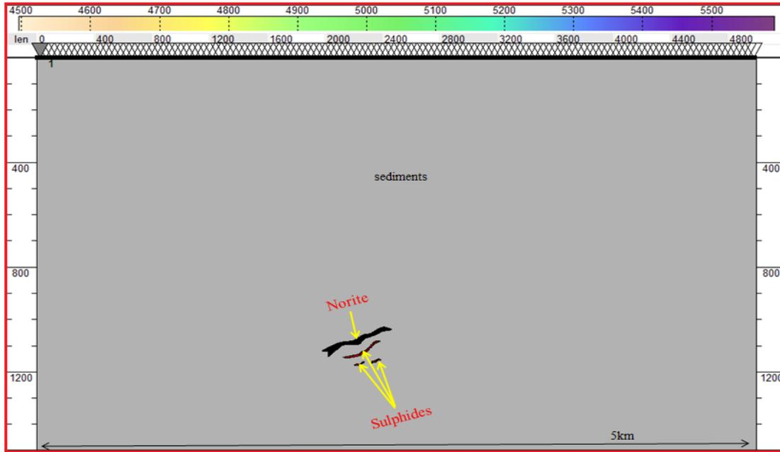
**Figure 1:** Synthetic 2D geology model showing the location of sulphides, norite and a sediment host rock.
