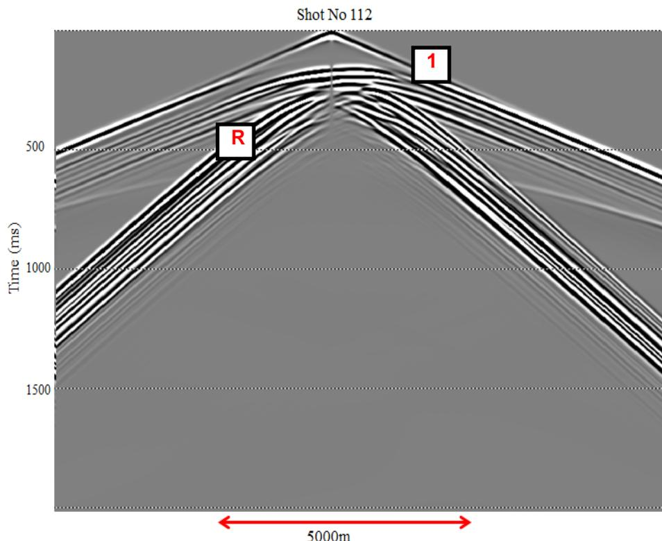
**Figure 3:** Synthetic shot records for source number 112 from the geological model (1) is the direct arrival signals, (R) is the reflections signals. The shot is displayed using true relative amplitude without correction for spherical divergence. Shot depth for all gathers is 0 m.
