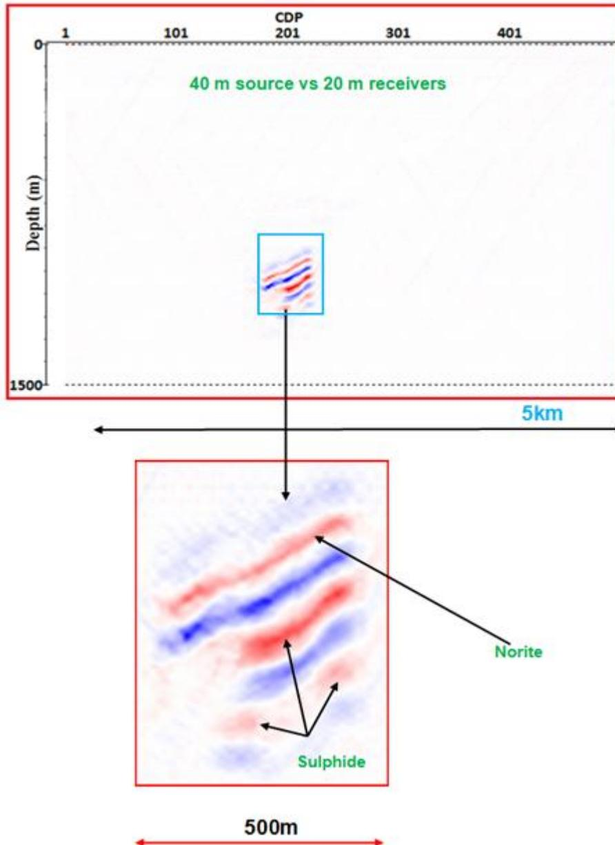
**Figure 5a)** Depth migrated sections with 40m source and 20 m receivers spacing 4b) Expanded section of the massive sulphide region in the model. Arrows in the expanded section indicate reflections from sulphides and norite.
