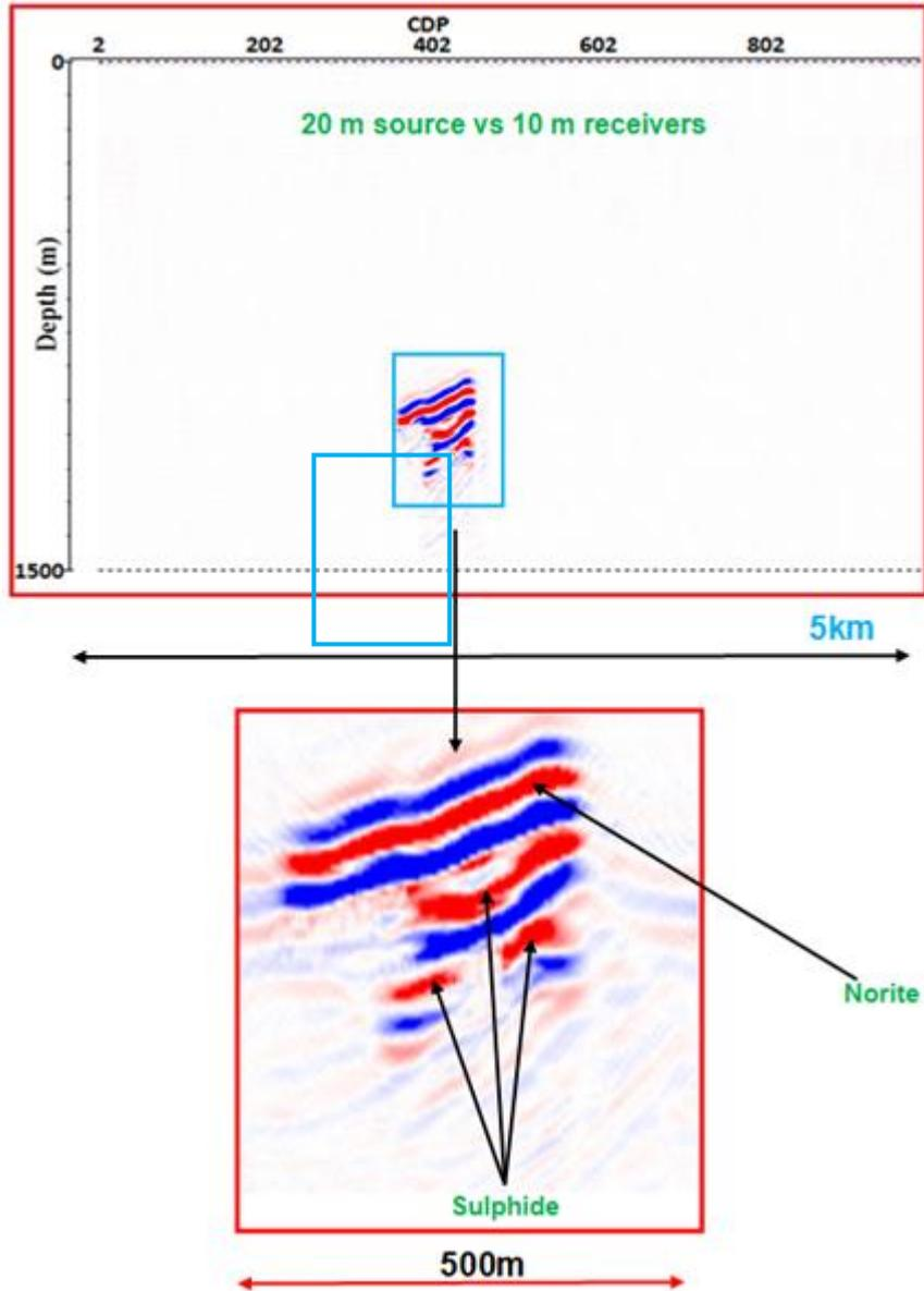
**Figure 4a)** Depth migrated sections with 20m source and 10 m receivers spacing 4b) Expanded section of the massive sulphide region in the model. Arrows in the expanded section indicate reflections from sulphides and norite.
