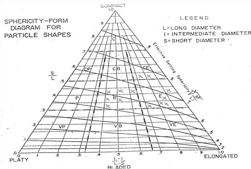
**Fig 3: Sphericity – form diagram for the particle shapes**
