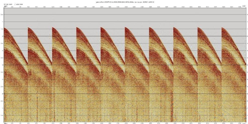
Fig. 2a: Data before application of swell noise attenuation processes.
