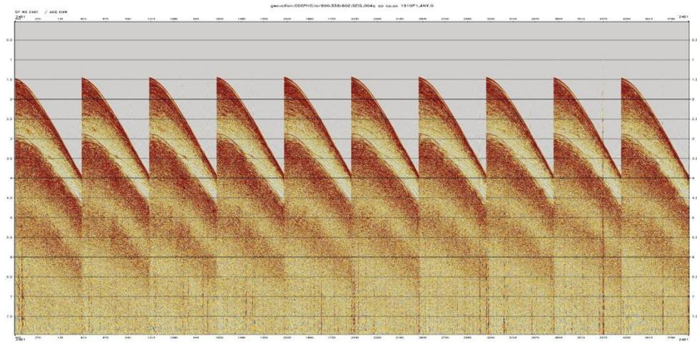
Fig. 1a: Data before application of swell noise attenuation processes.
