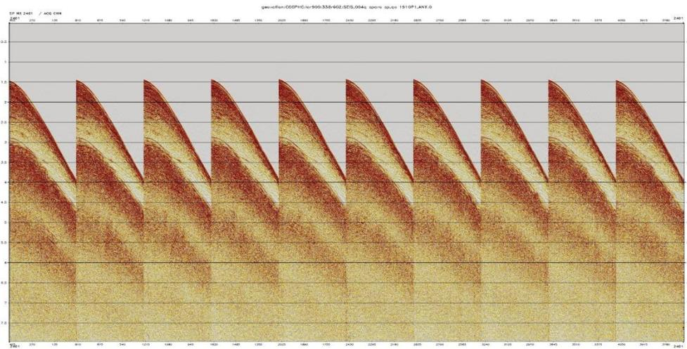
Fig. 1b: Data after application of swell noise attenuation processes
