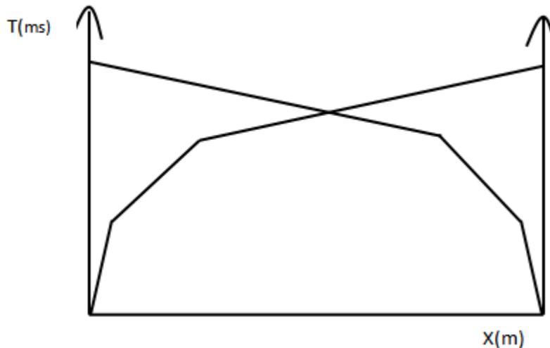
Fig. 2: Typical P-wave T-X curve obtained at the study area
