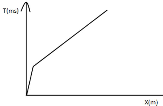
Fig. 3: Typical S-wave T-X curve obtained at study area.
