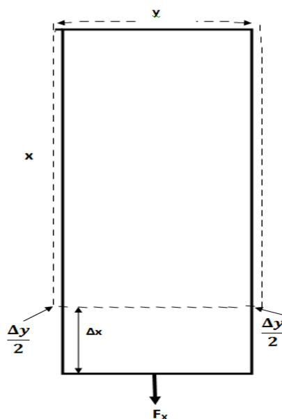
**Fig. 1.** Shape deformation of a rectangular bar due to the action of a tensile force.
