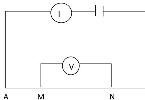
**Fig 1:** Schematic diagram of schlumberger electrodes array.
