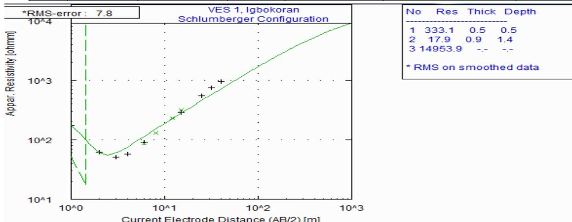
Fig 6: Typical Vertical Electrical Sounding Curve and Model Parameters.
