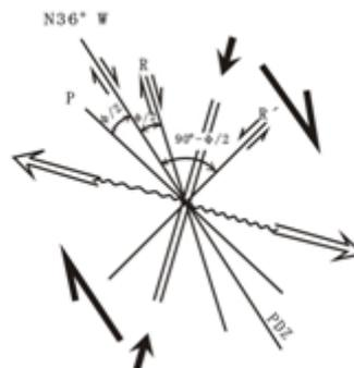
Fig 2. Riedel model of dextral simple shear
