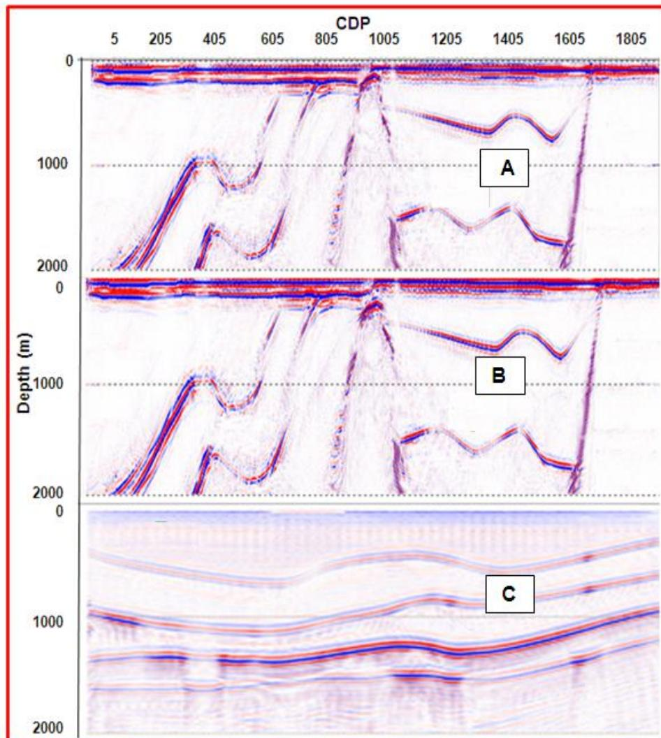
**Figure 5:** Migrated section: Panels (a), and (b) show the effect of different survey paarmeters in imaging the intrusive near the fault boundary (tight vs sparse). Panels (c) is the migrated section of non intrusive structure (only metasediments). In panels (a) and (b), the top of the intrusive can be detected near the fault.
