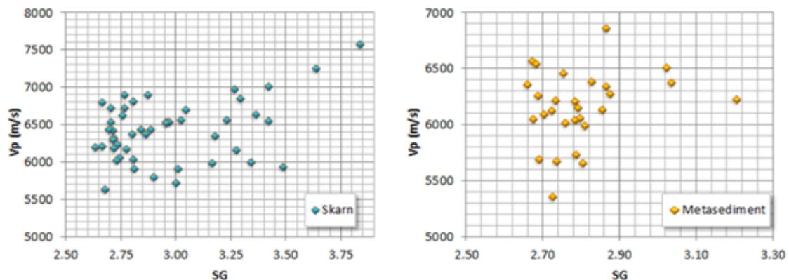
**Figure 2:** Scatter plot of specific gravity vs. P-wave velocity data measured from the core samples from Hillside Cu-Au Mining project
