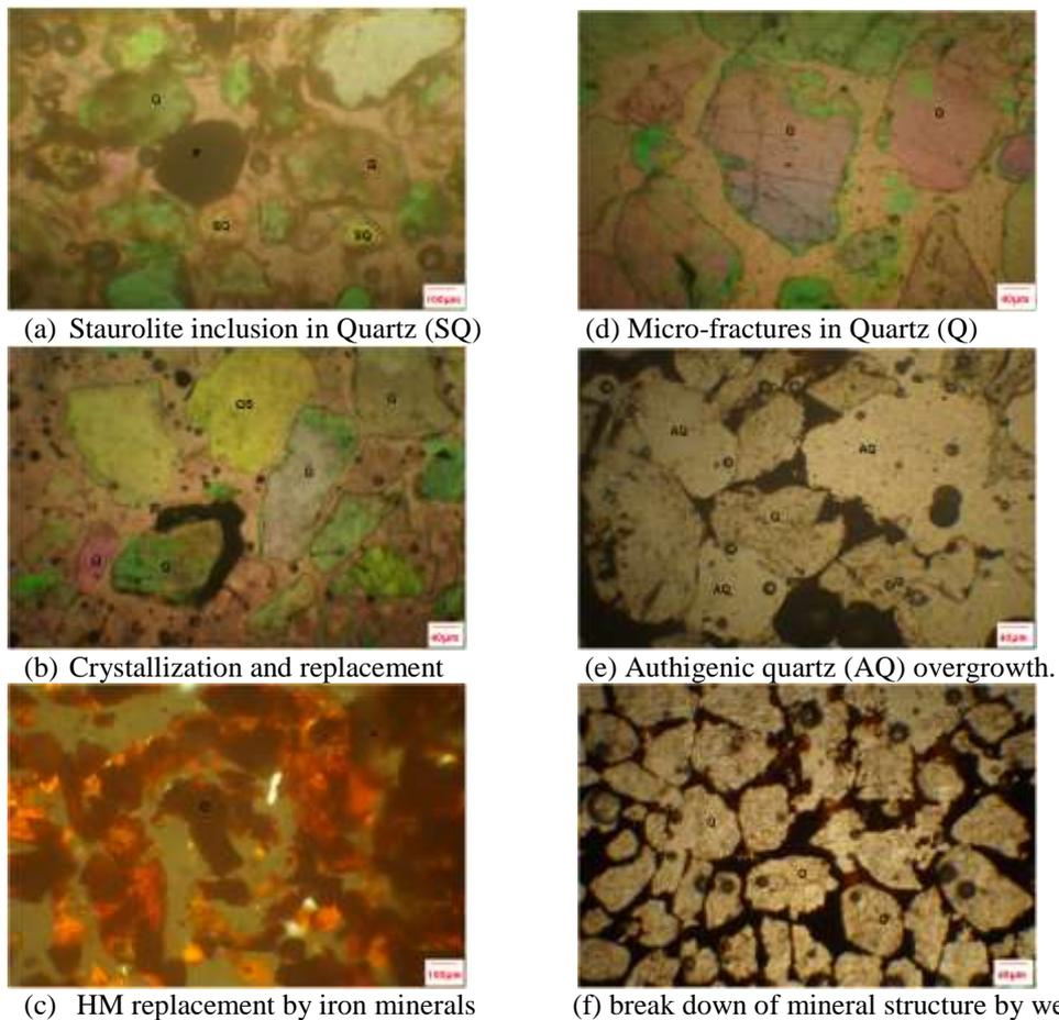
Figure 4: Photomicrograph showing the typical diagenetic process in Eocene sands of Upper Ameki Group. (HM=Heavy minerals)
