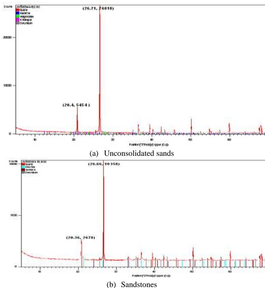
Figure 5: Typical minerals identified using XRD pattern for Eocene sands of Upper Ameki Group.
