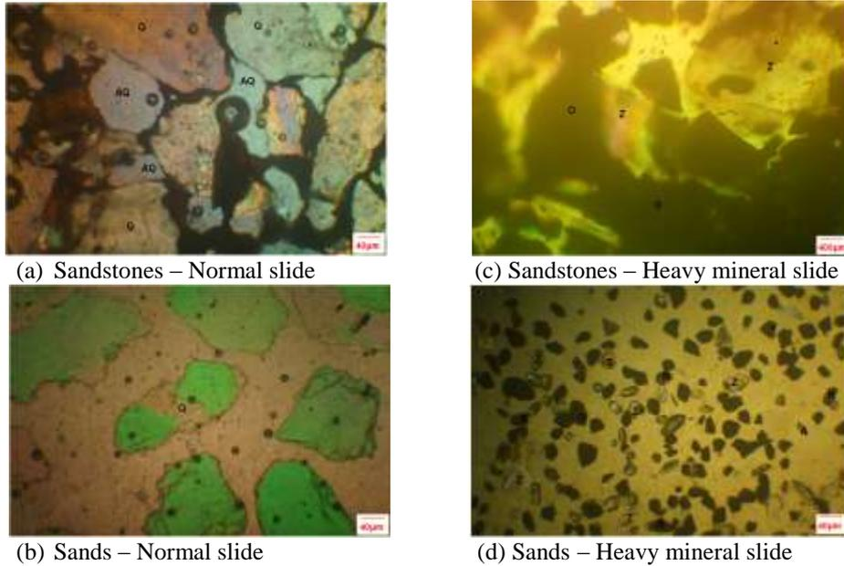
Figure 3: Photomicrograph of Eocene sands of Ameki Group. Note: Authigenic Quartz (AQ), Quartz (Q), Zircon (Z), Rutile (R), Tourmaline (T) and Opaque (O).
