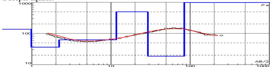
Figure 4.6d: Resistivity (Ωm) against AB/2 (m); Transect 4 VES Station 4.
