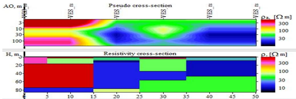
Figure 4.3c: Pseudo Cross-section and Resistivity section, Transect 5 VES 1, 2, 3 and 4
