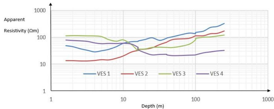
Figure 4.1a: Apparent Resistivity curves against depths for transect 1.
