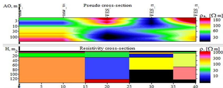
Figure 4.3a: Pseudo Cross-section and Resistivity section, Transect 2 VES 1, 2, 3 and 4
