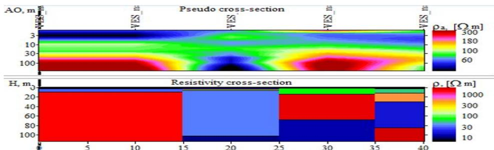
Figure 4.3b: Pseudo Cross-section and Resistivity section, Transect 4 VES 1, 2, 3 and 4
