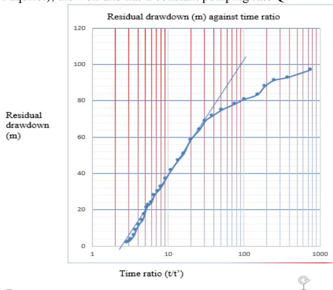
Figure 4.7: Residual Draw down (m) against Time Ratio.
