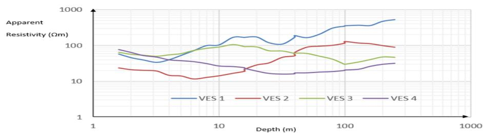
Figure 4.1b: Apparent Resistivity curves against depths for transect 2.
