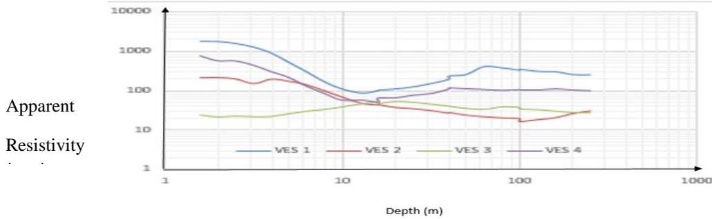
Figure 4.1d: Apparent Resistivity curves against depths for transect 5.
