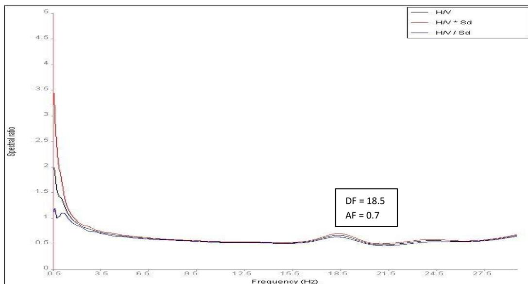
Figure 6. Value of dominant frequencies and amplification factor at Maitri Seismic Site.
