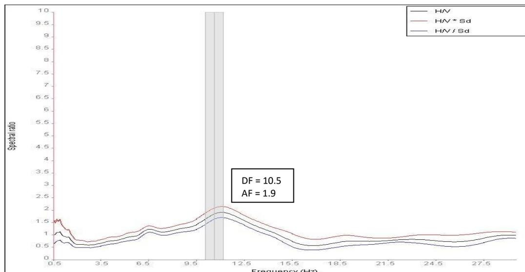
Figure 7. Value of dominant frequencies and amplification factor at Hyderabad Seismic Site.
