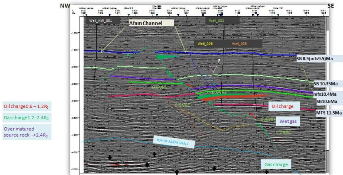
Figure 6: Diagram showing the generation, accumulation and migration of the hydrocarbon charge in the study area.
