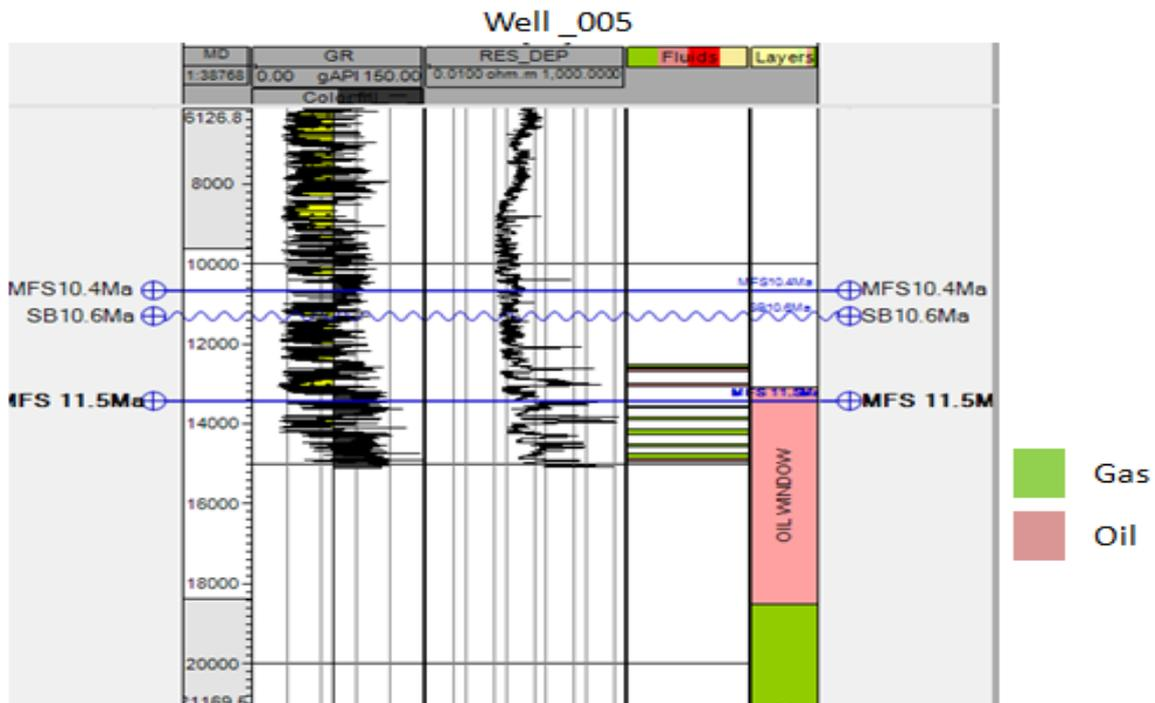
Figure.4: Well 005 showing the comparison of the hydrocarbon contacts in the field to the predicted charge(layers).
