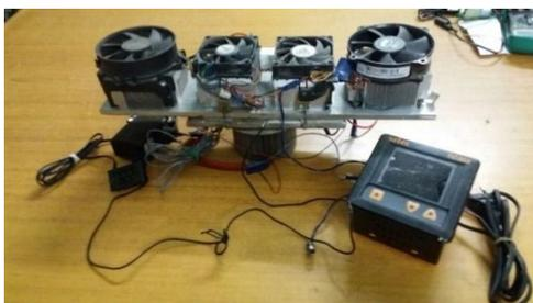
Fig:4 Experimental set up of thermoelectric generator with cooling fans and heat sink.
