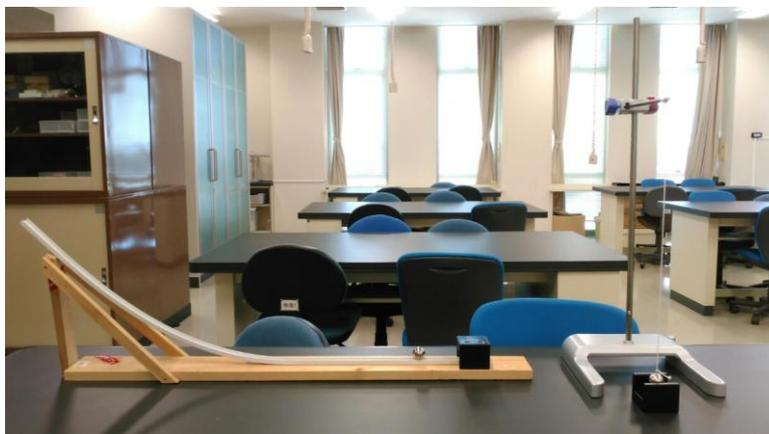
Figure 1: Set up of the experiments (left: inclined rail, right: pendulum).
