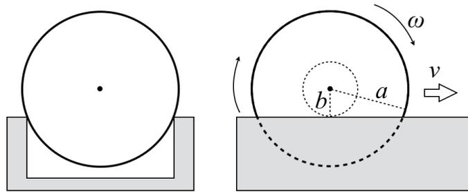
Figure 2: The ball rotating on the rail.
