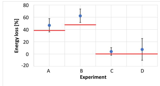
**Figure3:**Energy loss  $\epsilon$  of Eq. (2.7) for each experiment with  $3\sigma$  error bars. Horizontal red lines are theoretical values  $\epsilon_{th}$  shown in Table 1.
