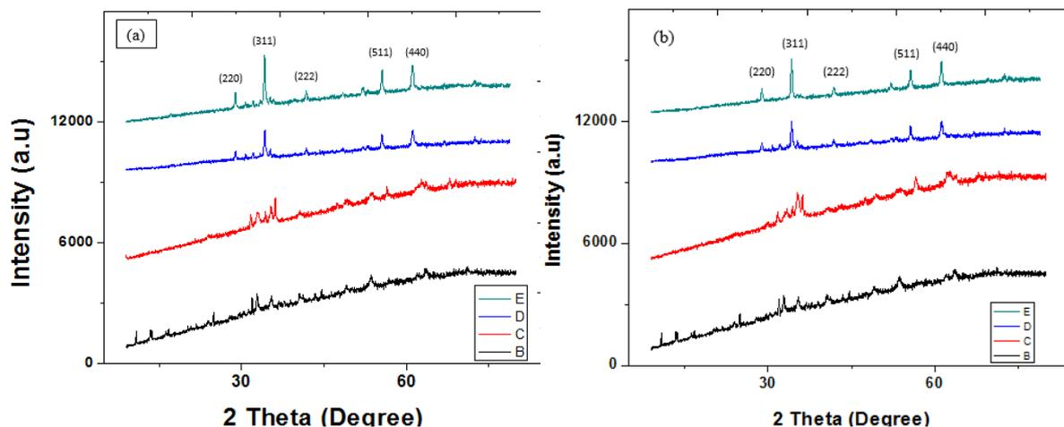
**Figure 2.** XRD patterns of ZF NPs (a) 0.1g and (b) 0.2g calcined at 0 and 500<sup>o</sup>C where (B is ZF only\_unannealed, C is ZF capped PVA\_unannealed, D is the ZF only\_annealed and E is the ZF capped PVA\_annealed)
