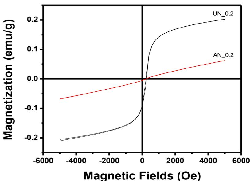
**Figure 3.** Magnetization curves for ZFNPs as prepared and at 500<sup>o</sup>C
