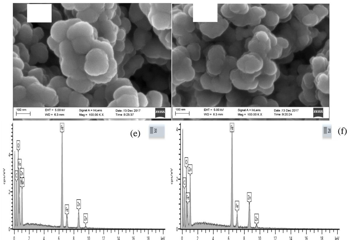
**Figure 1.** SEM images of Zinc ferrite nanoparticles capped with PVA Un-annealed (a) 0.1g (b) 0.2g and the annealed (c) 0.1g (d) 0.2g. The EDX images are shown in (e) 0.1g and (f) 0.2g
