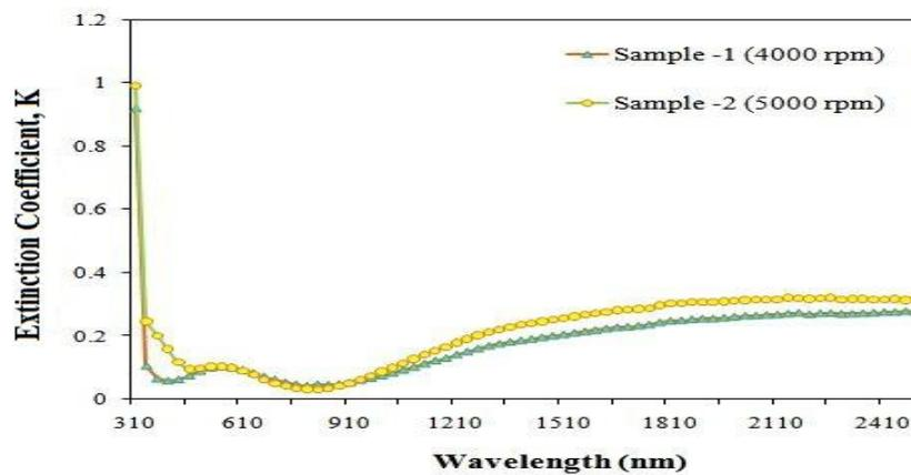
Figure 8. Extinction co-efficient of AZO samples (different rpm) vs. wavelength
