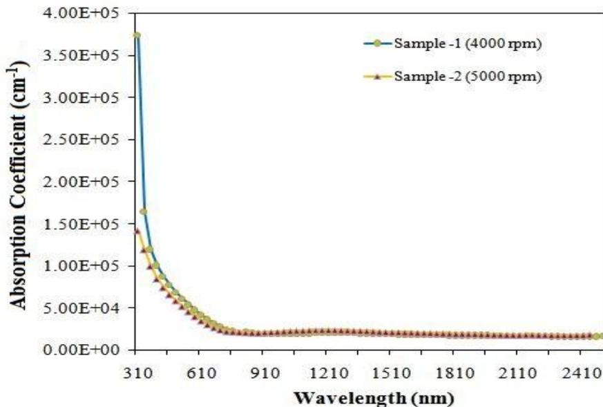
**Figure 6.** Absorption co-efficient of AZO samples (different rpm) vs. wavelength
