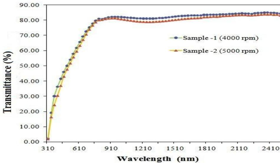
**Figure 5.** Optical transmittance of AZO thinfilms
