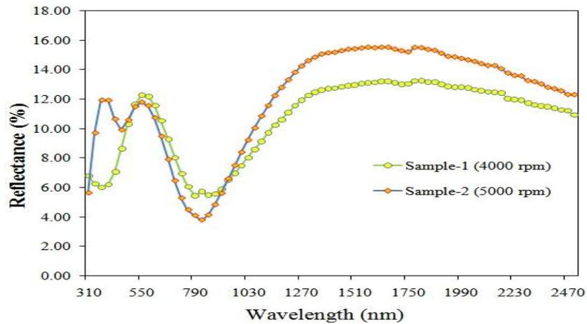
**Fig 3:** Reflectance (%) of AZO samples (different rpm) with respect to wavelength
