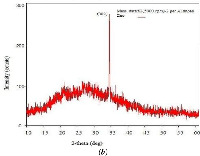
Figure 1. XRD pattern of AZO thin film for (a) Sample-1 (4000 rpm) and (b) Sample-2 (5000 rpm)
