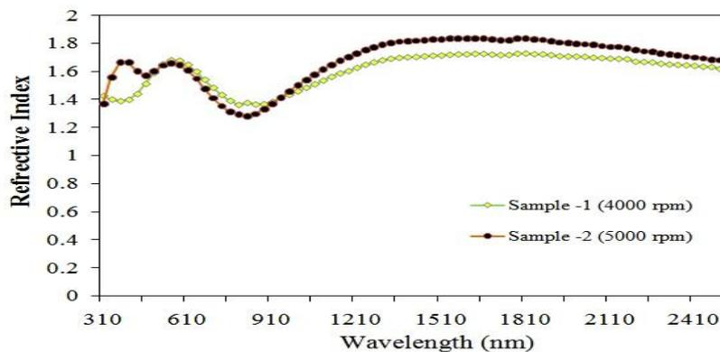
Figure 9. Refractive index of AZO samples (different rpm) vs. wavelength
