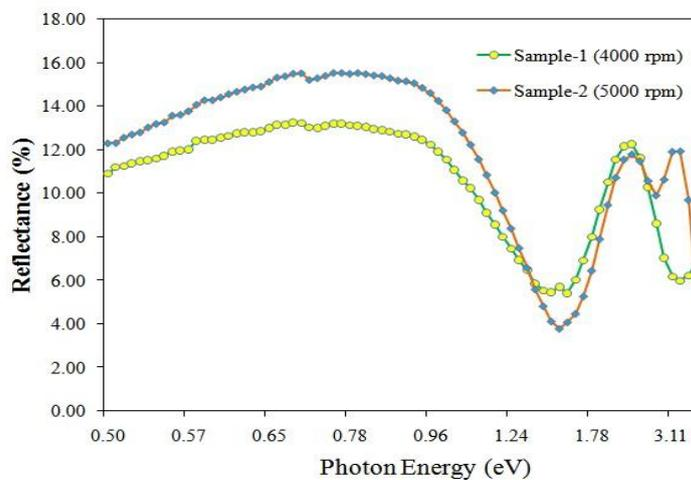
**Fig 4:** Reflectance (%) of AZO samples (different rpm) with respect to photon energy
