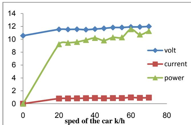
Figure no 3: The speed against the volt, current and power for third fan
