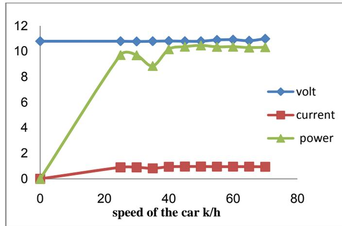
Figure no 5: The speed against the volt, current and power for fifth fan
