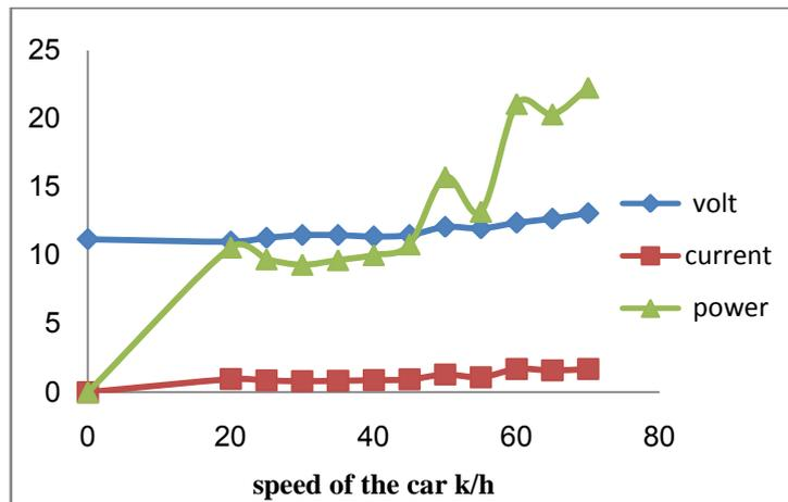
Figure no 4: The speed against the volt, current and power for fourth fan
