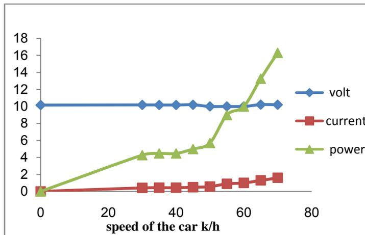
**Figure no1:** The speed against the volt, current and the power progressively for first fan
