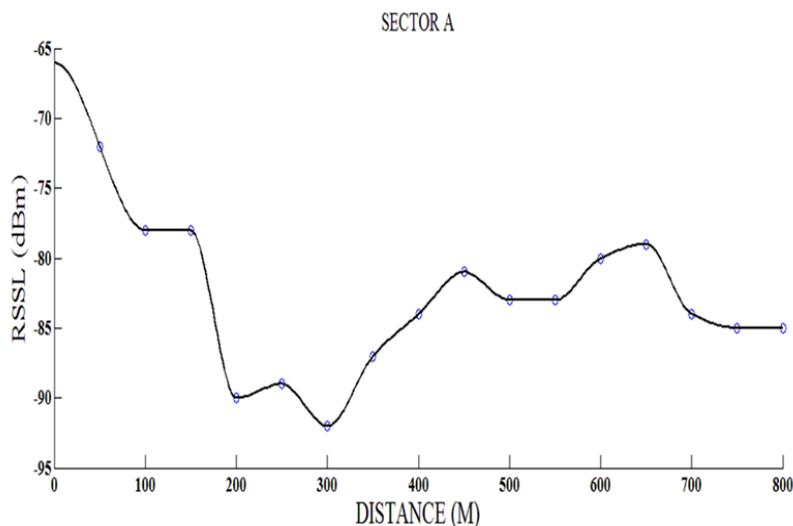
**Fig. 2:** Graphical representation of the Unfiltered Received Signal Strength of Sector A.
