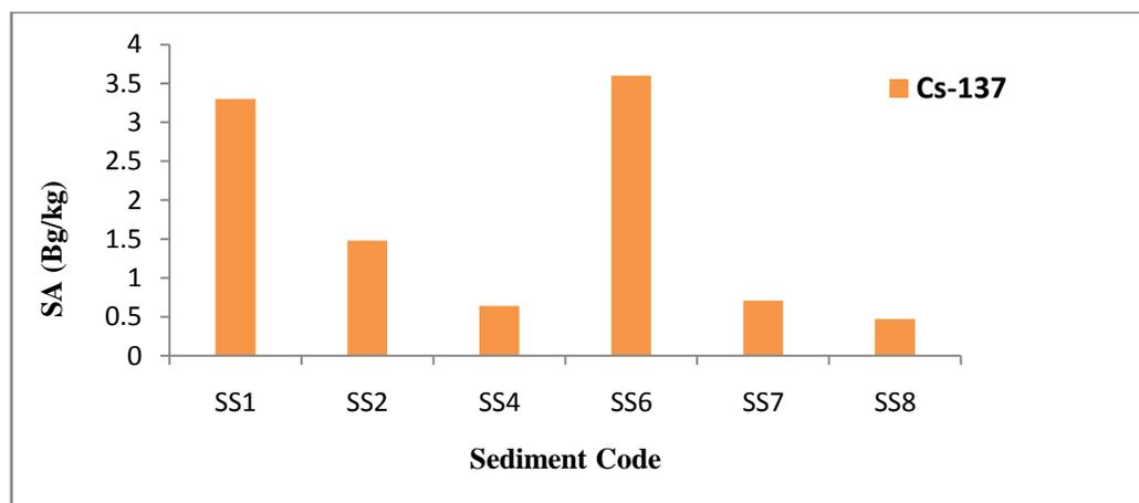
**Fig.4:**The radiological specific activity (SA) of Cs-137 isotope as a function of sedimentsample location
