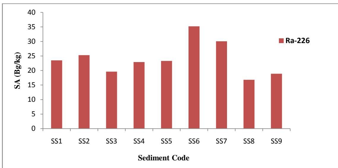
**Fig.1:**The radiological specific activity (SA) of Ra-226 isotope as a function of sediment sample location
