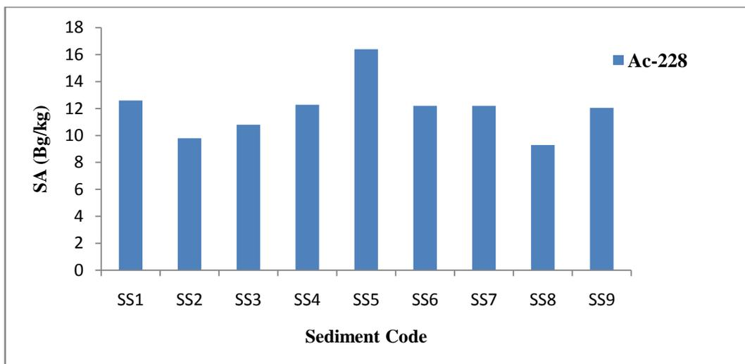
**Fig.2:** The radiological specific activity (SA) of Ac-228 isotope as a function of sediment sample location
