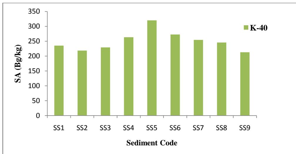
**Fig.3:** The radiological specific activity (SA) of K-40 isotope as a function of sedimentsample location
