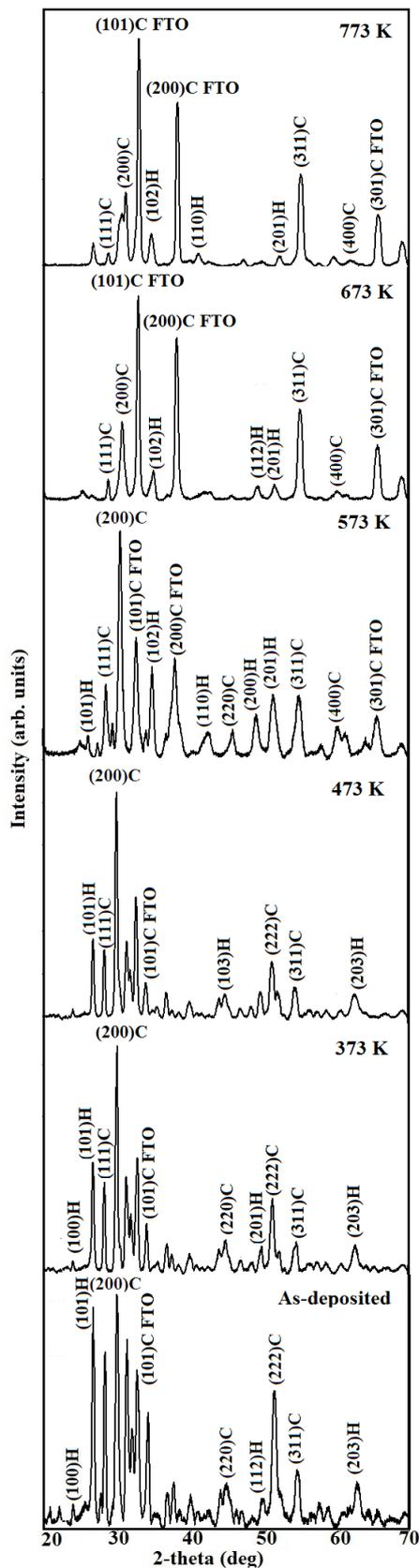
Figure 3. X-ray diffractograms of the CdSe/FTO nanowires as-deposited and annealed in air atmosphere.
