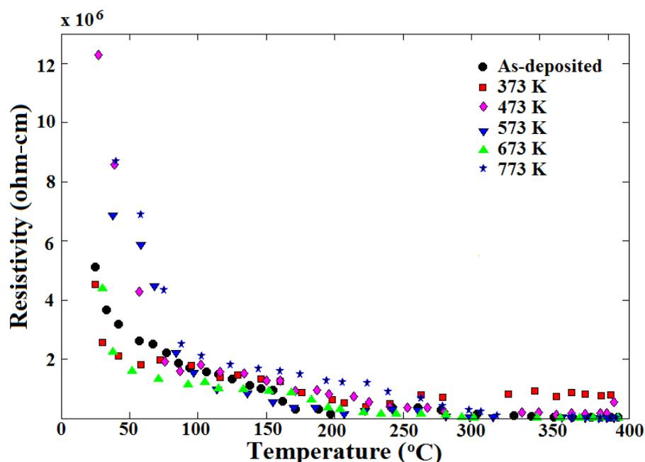
**Figure 5.** The temperature dependence of the electrical resistivity of the CdSe/FTO nanowires as-deposited and annealed in air atmosphere.
