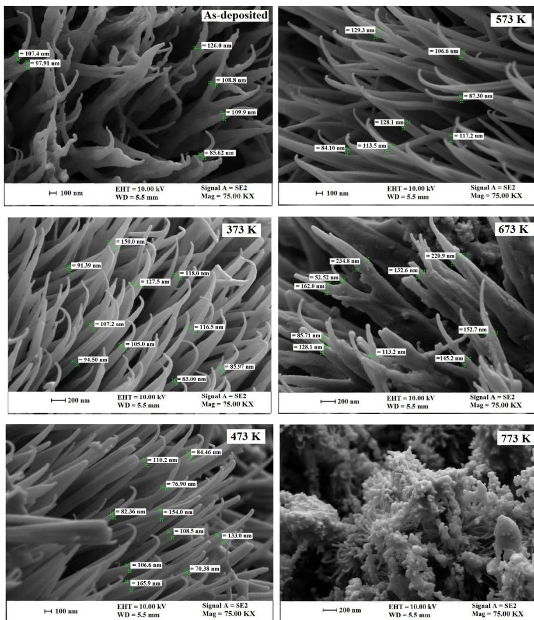
**Figure 2.** SEM images cross-sectional surfaces of the CdSe/FTO nanowires (a) as-deposited, and annealed in air atmosphere at (b) 373 K, (c) 473 K, (d) 573 K, (e) 673 K, (f) 773 K.
