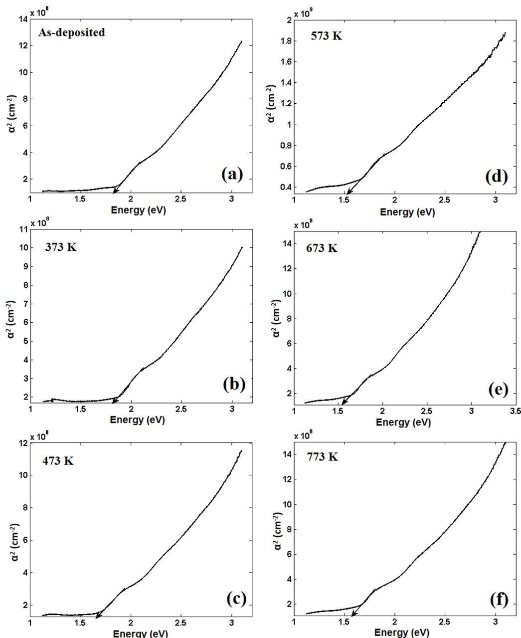
**Figure 4.** The  $\alpha^2$  versus  $h\nu$  for the CdSe/FTO nanowires as-deposited and annealed in air atmosphere at (b) 373 K, (c) 473 K, (d) 573 K, (e) 673 K, (f) 773 K.
