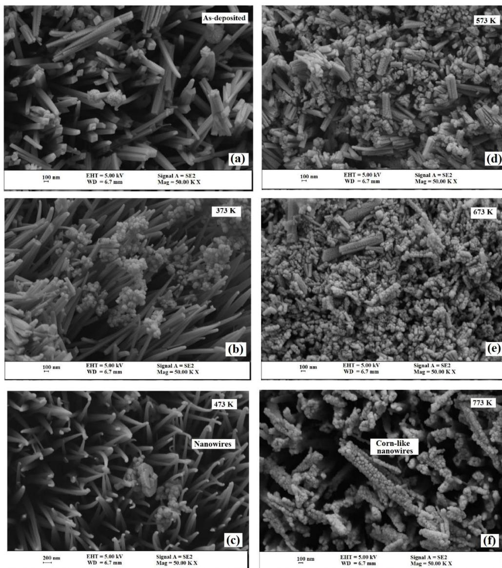
**Figure 1.** SEM images top surfaces of the CdSe/FTO nanowires (a) as-deposited, and annealed in air atmosphere at (b) 373 K, (c) 473 K, (d) 573 K, (e) 673 K, (f) 773 K.
