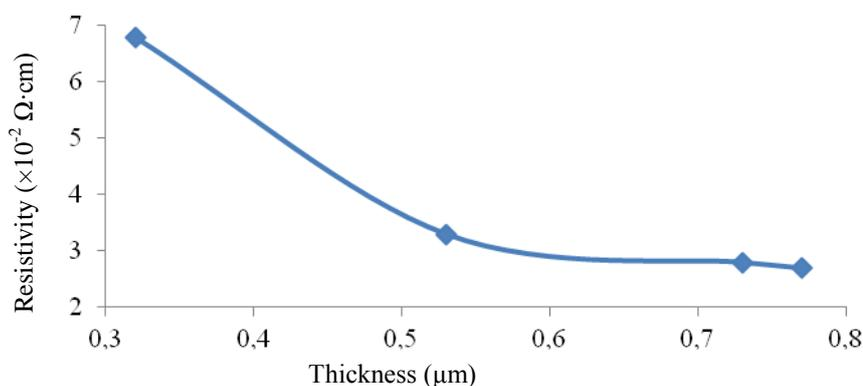
**Figure 1.** Variation of resistivities of some CIS thin films with respect to thickness
