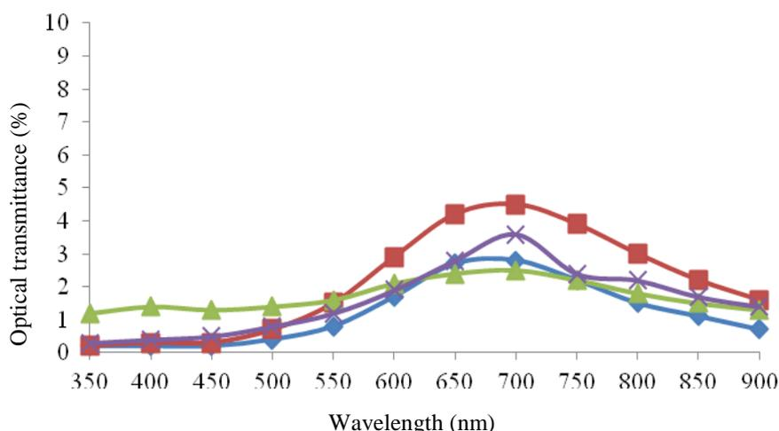
**Figure 2.** Variation of optical transmittance of some CIS thin films according to wavelength
