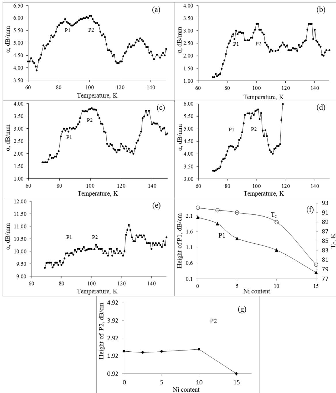
Fig. 5: The attenuation measurements of the ultrasonic longitudinal waves at frequency 4MHz for samples (a) Y123, (b) 2.5, (c) 5, (d) 10, (e) 15 wt.% Ni, (f) height of peak P1 &  $T_C$  vs. Ni content and (g) height of peak P2 vs. Ni content.
