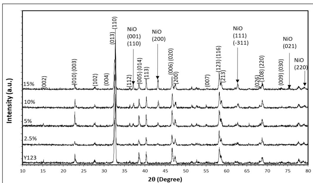
: XRD Patterns of (100-x) Y123 + x Ni samples ( $x = 0, 2.5, 5, 10, 15 \text{ wt.}\%$ )
