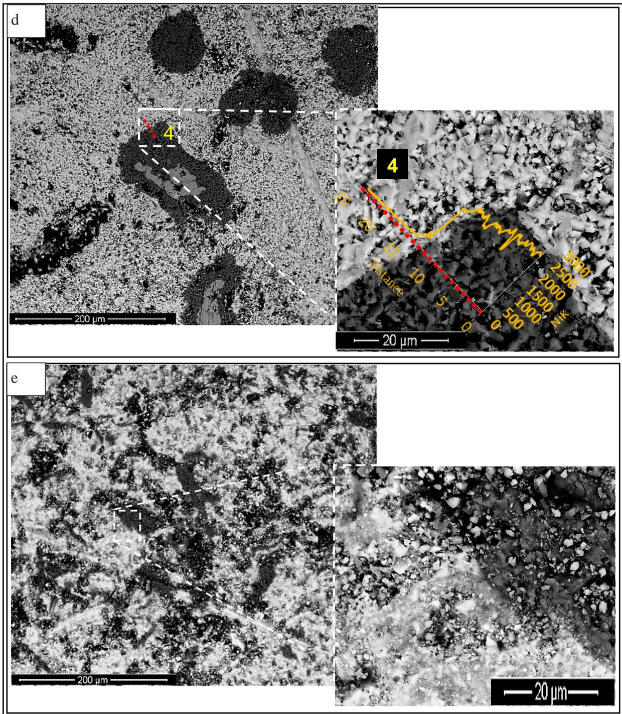
Fig. 3: SEM micrographs of the samples Y123 + x Ni composites (x = 0, 2.5, 5, 10 and 15 wt.%) marked as (a), (b), (c), (d) and (e) respectively and EDX analysis of Y123 and 2.5 wt.% Ni samples at positions marked as, X1, X2, X3 in addition to linear EDX analysis of 10 wt.% Ni sample at line marked as \4.
