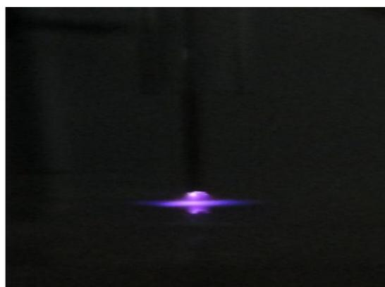
**Figure 2:** Camera view of atmospheric pressure NPDBD plasma.
