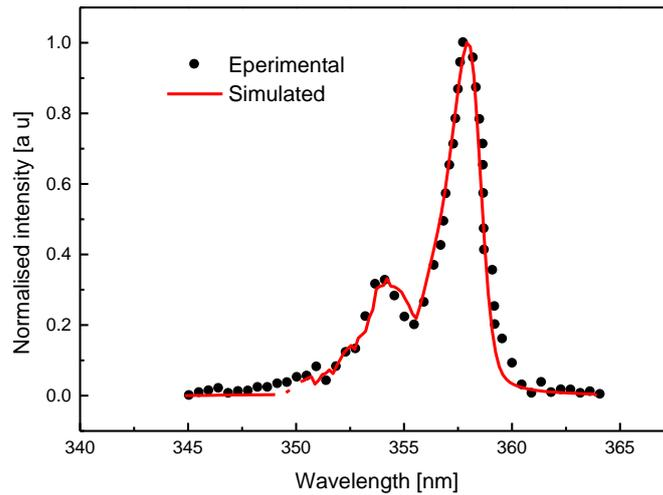
**Figure 4:** LIFBASE fitted nitrogen band for 1.0 mm air gap with 0.15 mm dielectric (glass) thickness.
