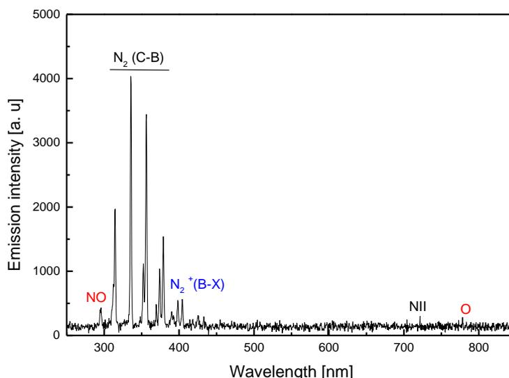
**Figure 3:** Emission spectra of 1.0 mm air gap and 0.45 mm dielectric thickness plasma with 5 kV source voltage and 20 kHz frequency.
