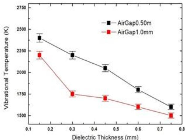
Figure 6: Variation of vibrational temperature with dielectric thickness.
