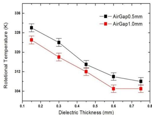
**Figure 5:** Variation of rotational temperature with dielectric thickness.
