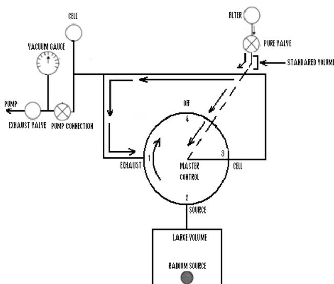
Figure 1: Experimental setup for the calibration of CN-85 SSNTD
