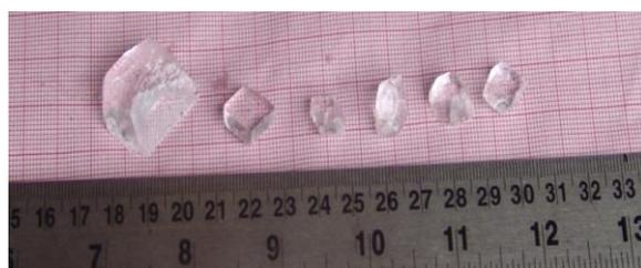
**Figure 1: Photograph showing the pure and urea added DSHP crystals grown [From left are : pure, 0.2, 0.4, 0.6, 0.8 and 1.0 mole% urea added]**
