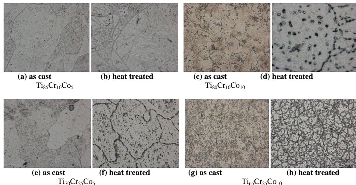
**Figure 2. Light micrographs of as cast and heat treated alloys (280x)**
