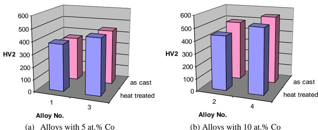
**Figure 4. Vickers hardness comparison of as cast and heat treated alloys**
