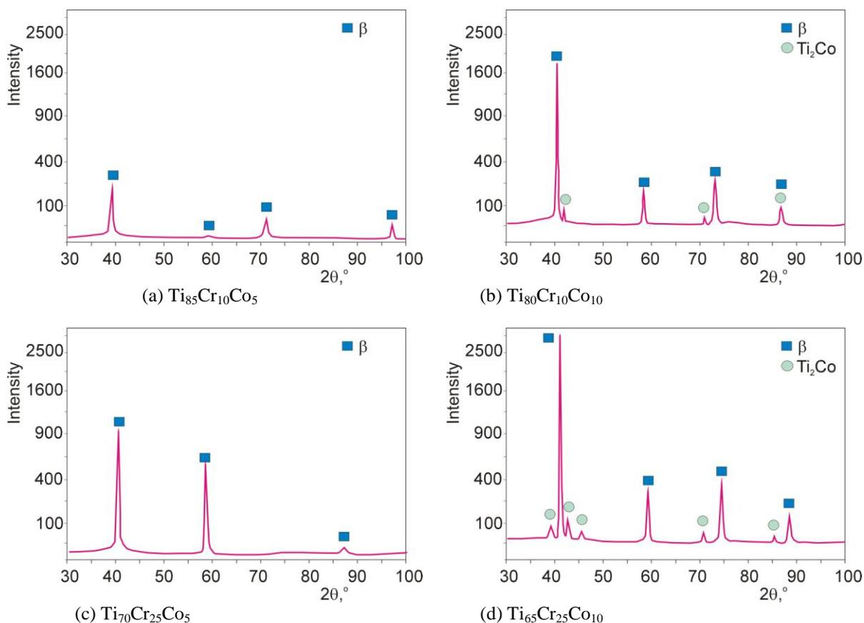
**Figure 1. XRD patterns of as cast experimental alloys**
